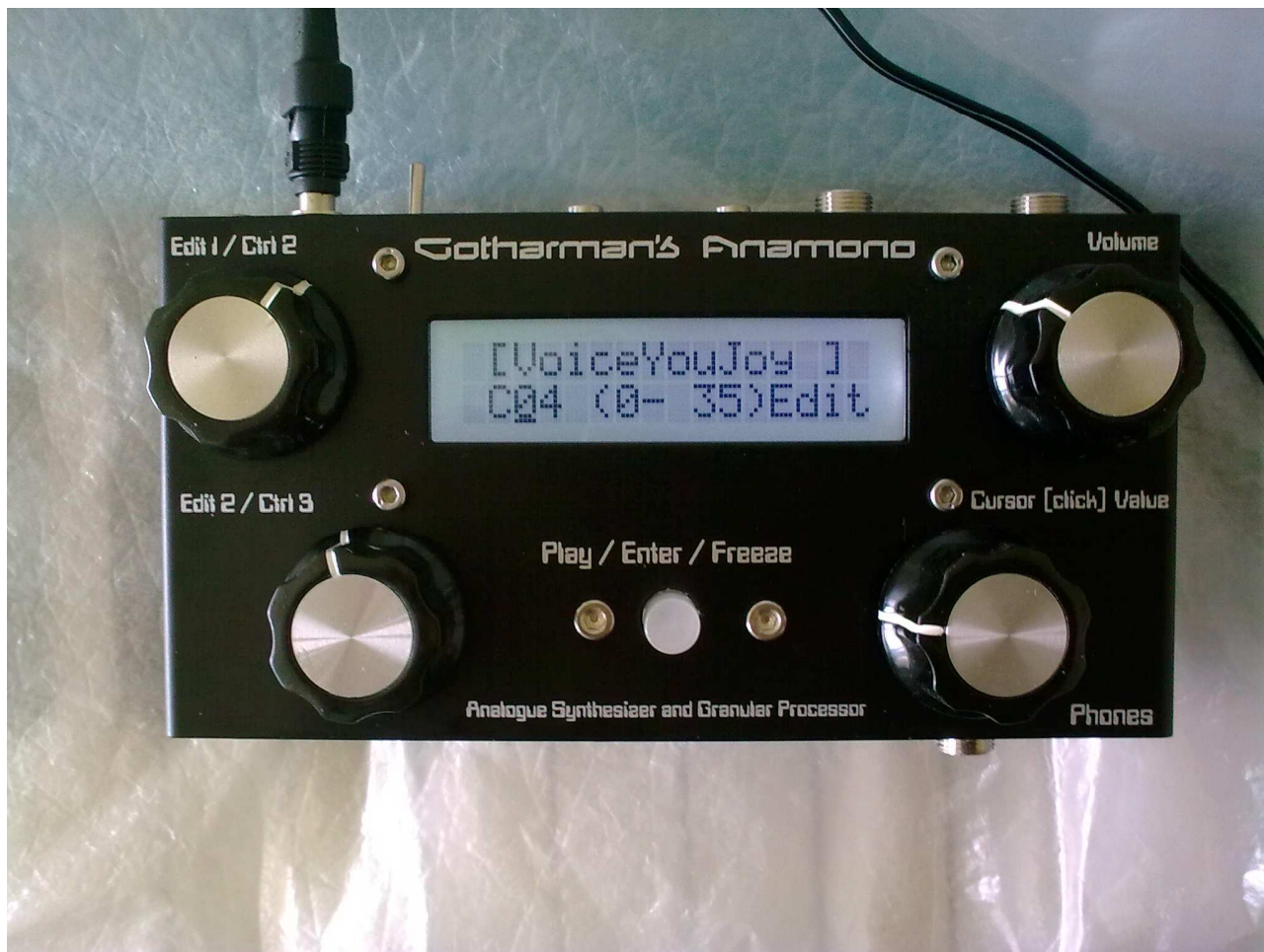
Analogue feedback synthesizer with build in granular processor
