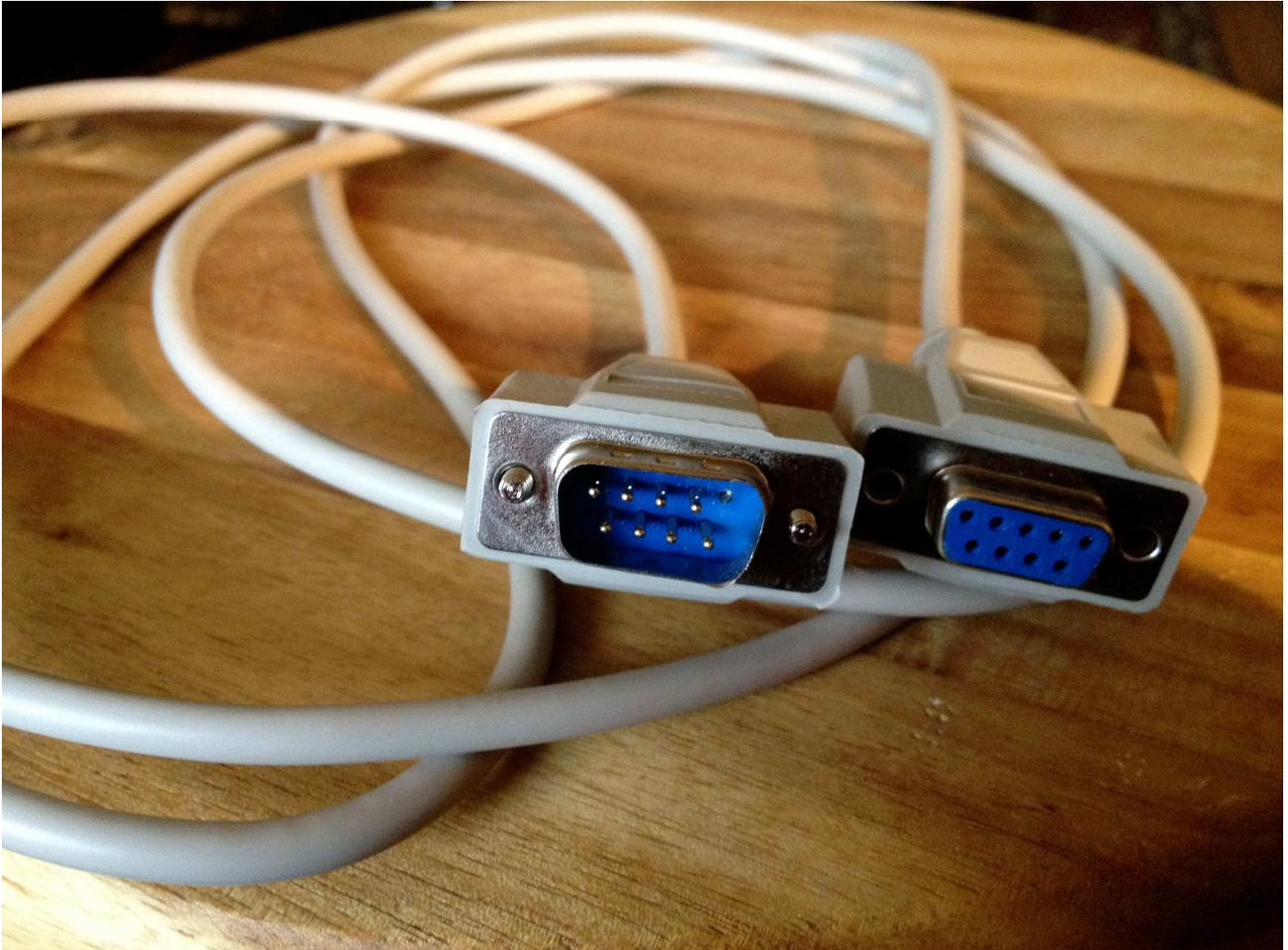
If you should need a longer cable, or if your cable one day gets lost, you can use a 1:1, 9-pin SUB-D cable. Just notice, that like on the picture, pin 5 of the male connector must be cut. This is because, on some Little deFormers, pin 5 on the expansion connector are connected to its audio path, and if this pin on the cable are connected, it will create a lot of noise on the audio.
