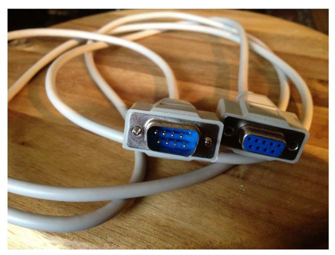
If you should need a longer cable, or if your cable one day gets lost, you can use a 1:1, 9-pin SUB-D cable. Just notice, that like on the picture, pin 5 of the male connector must be cutted. This is because, on some Little deFormers, pin 5 on the expansion connector are connected to its audio path, and if this pin on the cable are connected, it will create a lot of noise on the audio.
