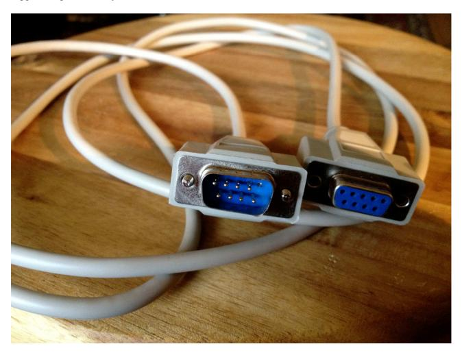
If you should need a longer cable, or if your cable one day gets lost, you can use a 1:1, 9-pin SUBD cable. If you have a Little deFormer 1, just notice, that like on the picture, pin 5 of the male connector must be cutted. This is because, on some Little deFormers, pin 5 on the expansion connector are connected to its audio path, and if this pin on the cable are connected, it will create a lot of noise on the audio. If you have a Little deFormer 2, you can just use the SUB-D cabel as it is.
