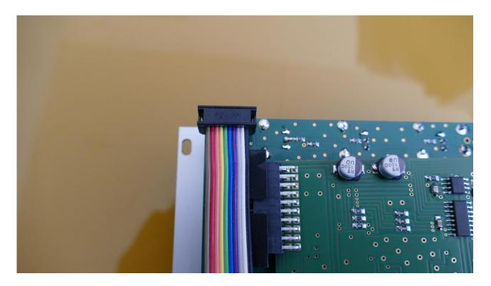
Connect the power cable with the brown cable (-12V) facing upwards, if it is a multi-colored cable, or the red line facing upwards, if it is a grey cable.
