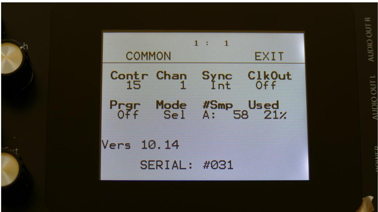
Here you must set the Mode parameter (MIDI In Mode) to either Omni, OmTh (Omni Thru), Mult (Multi-Timbral) or MuTh (Multi-Timbral/Thru). The CC control will not work properly in Sel (Selected) mode.
