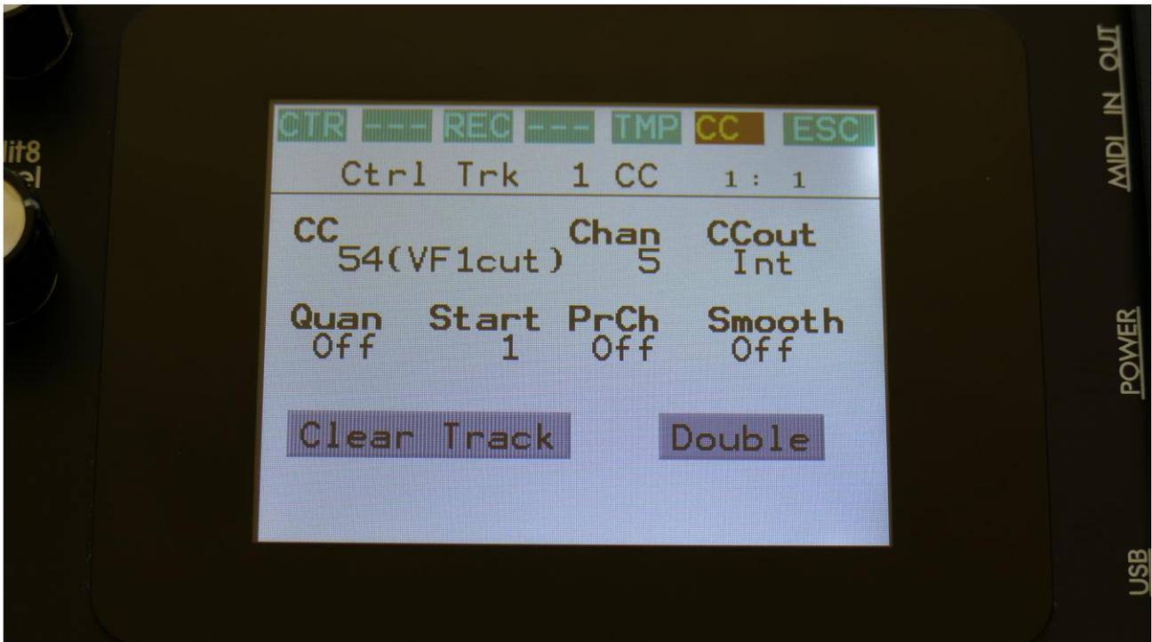
Set the CC parameter, to the parameter, that you want to control with the controller track. A shorted version of the parameter name, will be written in parenthesis.
