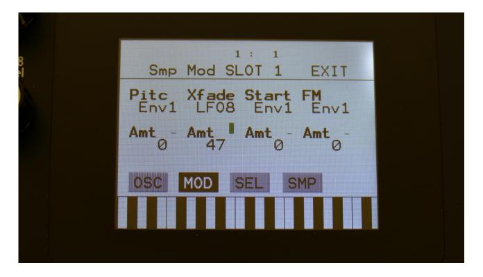
The **Chop** parameter on the sample oscillator MOD page, has been replaced by an **Xfade** parameter, to make it possible to modulate the crossfading.
