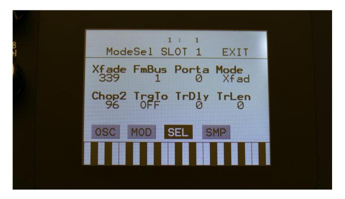
When switching to **Xfade** mode, the **#Smp** parameter will change its name to **Chop2**, and the **Xfade** parameter will become a numeric value.
