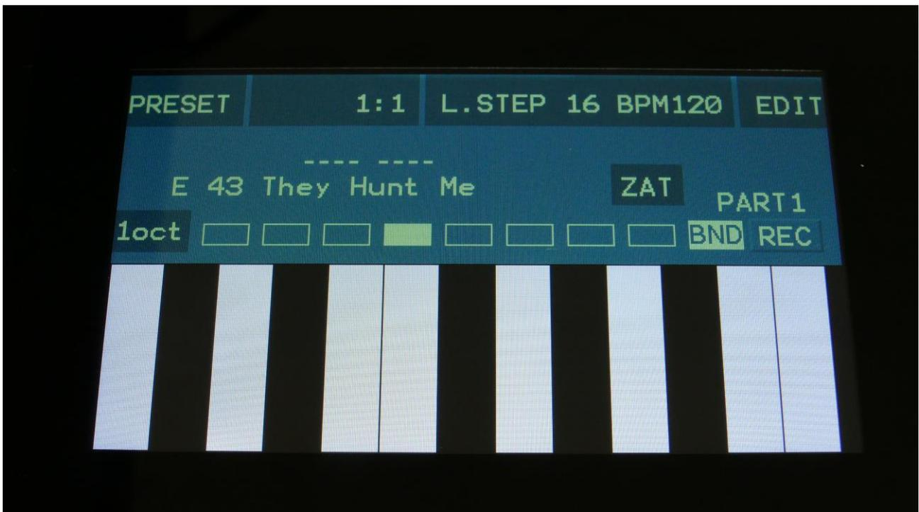
On the Preset Select page, zaTurn shows which filter board were installed, when the currently selected preset were saved, to make it easy to track, which filters were used for which presets. "ZAT" means that the original zaTurn filter board were installed, when this preset was saved.
