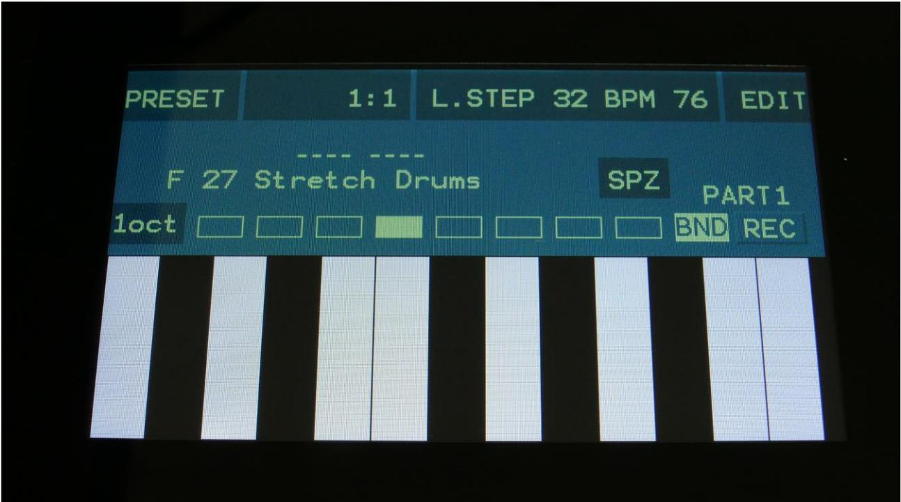
If the Spaze filters were installed, when a preset was saved, "SPZ" will be shown on the Preset Select page.
