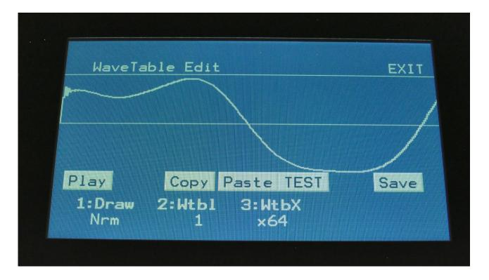
Here you can view and edit the wavetable one wave at a time. With **Edit Knob 2** you can select wave 1 to 8 or 1 to 64, depending on the wavetable mode. With **Edit Knob 3**, you can select the desired mode: **x8** (8 waves) or **x64** (64 waves).
