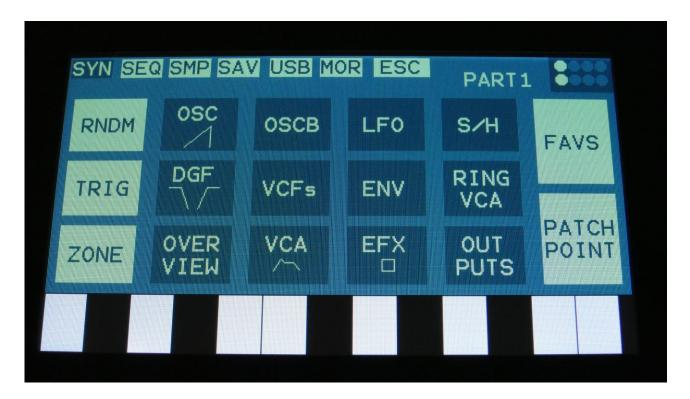
Here you have an overview of the different types of modules. To access a specific module, simply touch the module type, that you would like to enter. It is also possible to enter the modules by pushing the Modules/Bar Sel button, and then pushing a step button. Please see "Operating Zaturn", for more information about this.
