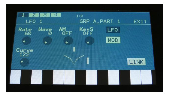
Each group has 4 LFO's (16 in total) with a waveform that morphs from triangle to sawtooth to pulse to FM waves. Curve can be adjusted from logarithmic to linear to exponential. The LFO's can be key synced, and a one-shot mode is available, for using the LFO's as envelopes. The Rate, Wave and Curve parameters can be modulated.
