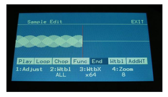
By touching the End touch button, so that it turns dark blue, the screen will now be focused on the end point, which is indicated as a vertical red line. When you touch the screen now, the red line will move, indicating that the end point is selected. It is also possible to change the end point, by rotating Edit Knob 1.
