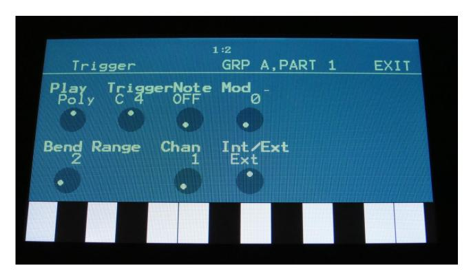
Select the part, that you would like to set up as internal or external, by holding down the Steps/part button, while pushing the step button, that has the desired part number.
