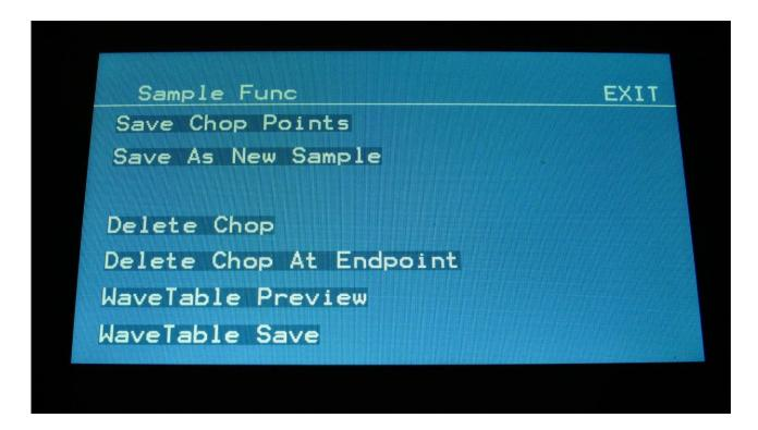
Touch **WaveTable Preview**, so that this turns white. Now you will hear your wavetable playing back. Adjust **Edit Knobs 1 and 2**, to scan through the waves (**Edit Knob 2** is only active at 64 waves).
