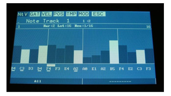
You can now, by turning Edit Knob 1, adjust the offset of all steps at the same time. Middle position of Edit Knob 1 is zero, above middle will turn the offset up, below middle will turn the offset down.
