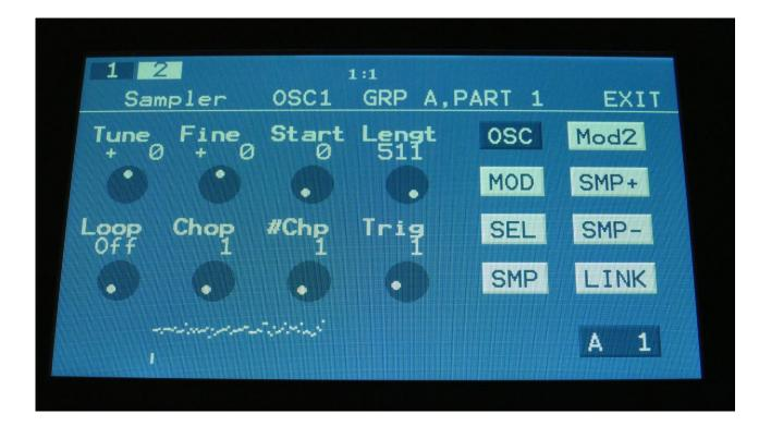
Set Loop mode to On, and adjust the Chop parameter, to select the single cycle waves. If you would like more single cycle waves to play back inside the loop, turn the #Chp parameter up.
