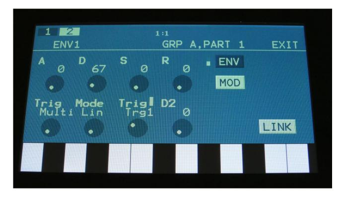
Each group has 2 envelope modules (8 in total), each with an ADSR envelope and a Decay envelope. The ADSR envelope can run in various linear and logarithmic modes, the envelope time can be timed by 4, for long envelope times, and the ADS segment can be looped. The envelopes can be trigged by any sources. The A, D, R and output amount parameters can be modulated. Envelope 2, the decay envelope, is always linear. When the ADSR Envelope is looped, the Decay envelope is looped in sync with this.
