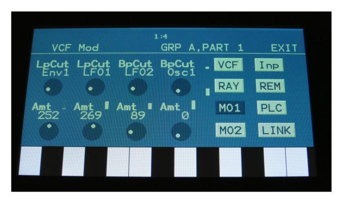
The "manual" way, is to go to a modules audio or modulation input pages, select the audio/modulation source, using Edit Knob 1 to 4, and adjust the amount/level, using Edit knob 5 to 8. Only positive sources can be selected this way. On modulation pages, you can touch the source select parameter, to change the source to negative.
