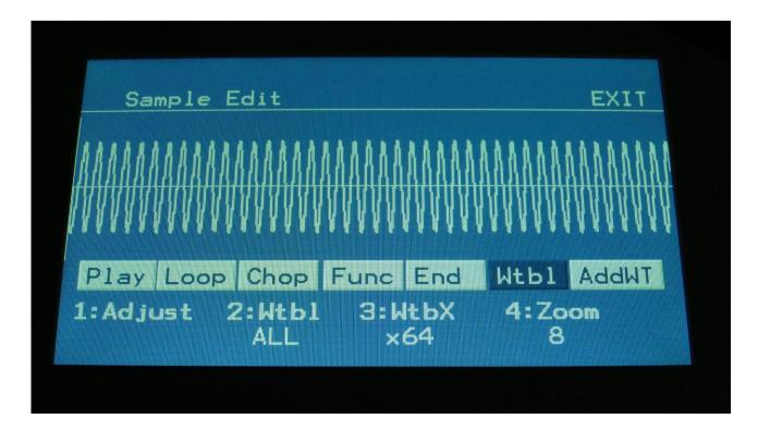
On the graphical sample edit page, with the sample, which you would like to build a wavetable from, selected, touch the Wtbl button, so that this turns dark blue. Zaturn will now create one wave for a table, consisting of 512 sample points, equally spaced between the selected start and end points. As soon as Wtbl mode is switched on, the currently generated wave will be audible.
