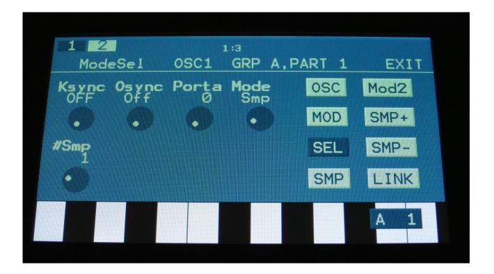
Set the Oscsillator in sampler mode, and touch the SMP touch button to select the sampling, that you just wave chopped (or any other sampling that you have wave chopped).
