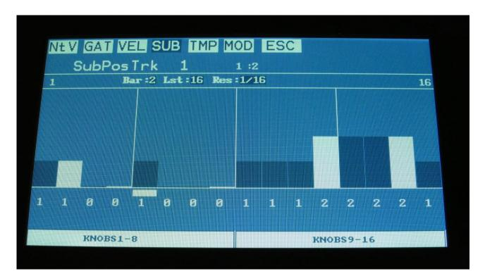
Here a value between 0 and 3 can be added to the step position for "micro-timing". A value of 0 will play back the step on the exact position. A value of 1 will delay the playback of the step by one quarter of the tracks resolution. A value of 2 will delay the playback of the step by one half of the tracks resolution. A value of 3 will delay the playback of the step by tree quarters of the tracks resolution.
