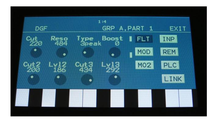
The 8 digital filters on Zaturn have 27 different filter types to choose from. Cutoff frequencies, resonance and triple filter levels can be adjusted and modulated.
