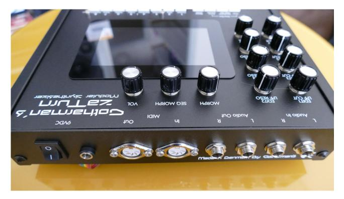
On the back panel of your Zaturn, you will find the power switch, connection for power supply, audio inputs and outputs and MIDI in and out.
