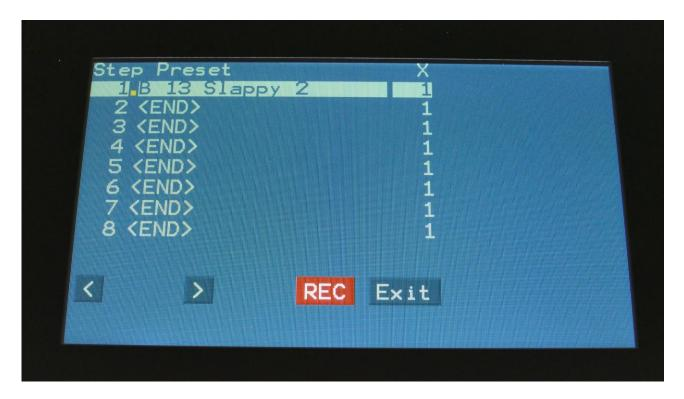
Make sure that the sequencer is stopped, and push the "REC" button, so it turns red.
