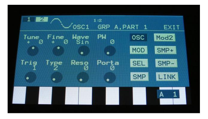
When you have entered a module type, that contains more than one of the same type, you can select the different module numbers, by touching the numbers in the upper left corner.
