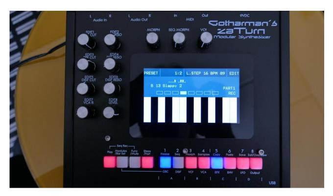
Zaturn has a highly sensitive and responsive capacitive touch display, 8 step/trigger/part select/quick jump buttons, a Modules/Bar Sel button, a Func/Mute button, a Steps/Part button and a Sequencer Play button. It has 8 Edit/Quick Edit Knobs for controlling and editing parameters and sending MIDI CC's, a (synth) Morph knob, a Sequencer Morph knob and a volume knob.
