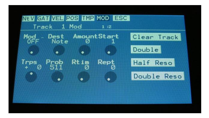
Here you can set up note track modulation, the track Note Randomizer, the start step, make step repeats, and transpose the track. It is also possible to clear or double the track, and it is possible to change the resolution of the track, without changing the timing.
