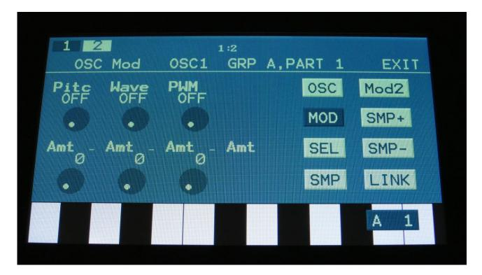
The small VU-meters next to the parameters, shows the activity of the selected modulation sources.
