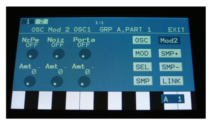
The Mod2 page, when Perc, Prc2 or Prc3 is selected as Type
