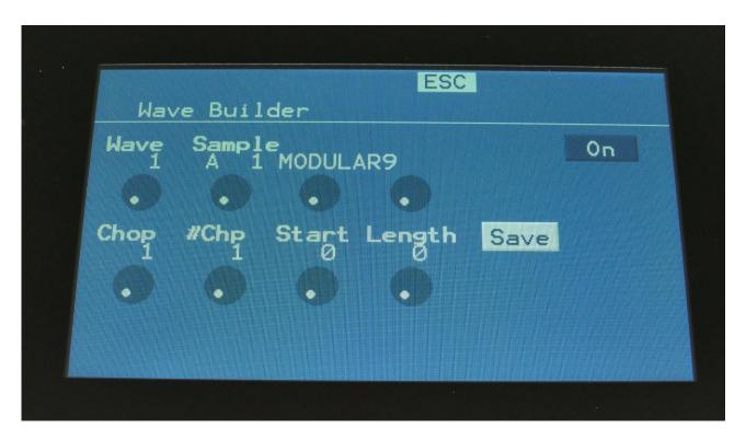
Wave: 1 to 8. Selects wave 1 to 8 of the wave sequence to be generated.
