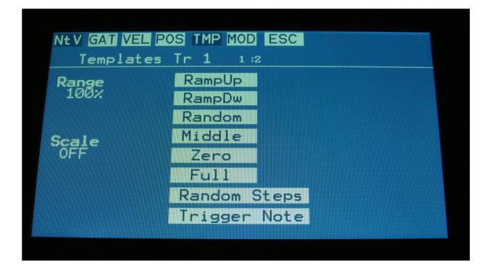
First turn Edit Knob 1, to set the range. This will set, how much the template routine will affect the values, that are already on the selected subtrack. When this is set to 100%, the template function will be absolute. Then touch any of the template boxes in the middle of the screen.
