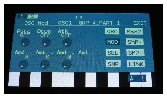
The MOD page, when Perc, Prc2 or Prc3 is selected as Type
