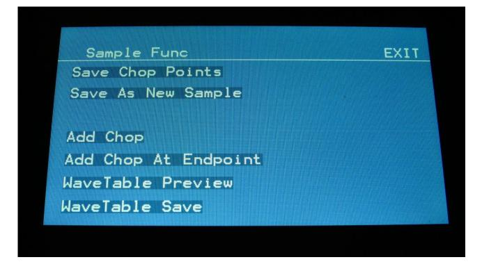
Touch "Save As New Sample". A new page will now open. Select the sample bank, that you would like to copy the sampling/portion of the sampling to, by touching the A, B, C or D touch button.
