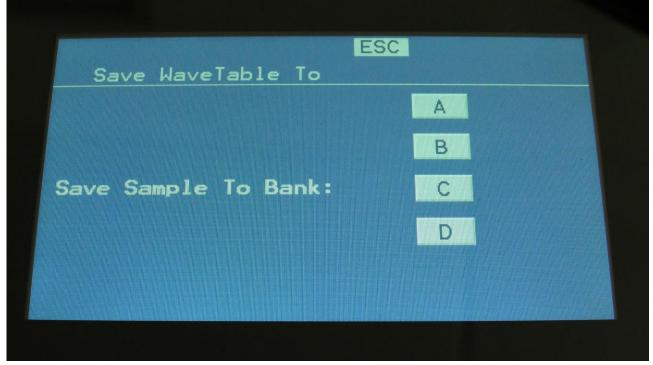
Select the sample bank, on which you would like to save the wavetable to, by touching the A, B, C or D field. 18 min. and 43 min. Zaturn's only has Bank A. Now the naming page will show:
