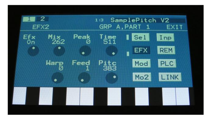
Zaturn has 8 effect processors, 2 in each group, EFX 1 and 2. All effect types are available in both EFX 1 and 2, but EFX 2 has some additional "large" effects, like reverb and granulators. Most parameters can be modulated. Zaturn has many of the classic deFormer effect, but also some new ones, like a wavefolder and some new pitch effects.
