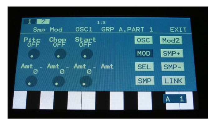
The MOD page, when in sampler or chopped keyboard mode
