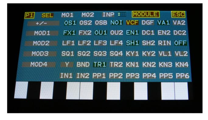
To connect modules on the overview page, first touch the SEL button in the top of this page. The SEL button should now turn brown. Then touch the module, for which you want to connect the modulation/inputs. This module will now turn brown. Then touch either the MO1 (modulation page 1), MO2 (modulation page 2) or INP (audio inputs) in the top of this page, depending on what you wish to connect.
