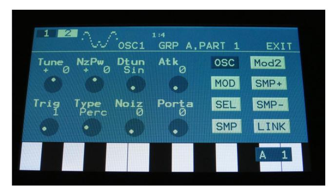
The OSC page, when Perc, Prc2 or Prc3 is selected as type
