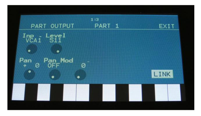
In the output module, signals from any modules can be assigned and routed to the audio outputs. Panning of sounds and pan modulation is also done here.
