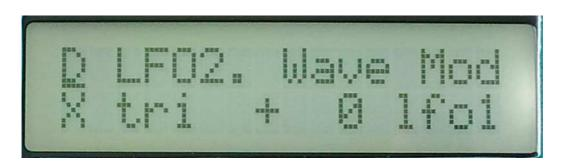
Edit 1: Oscillator LFO 2 waveshape. Value 0-255. 0: triangle, 64: saw, 128: square, 255: pulse.
