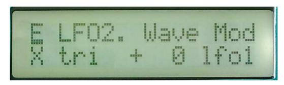
Edit 1: Filters LFO 2 waveshape. Value 0-255. 0: triangle, 64: saw, 128: square, 255: pulse.
