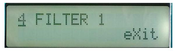
The deMOON has four filters which are indepenently programable and each can be routed in serial or parallel to the others. Each filter can be set in lo-pass, band-pass or hi-pass mode. Cut-off, resonance and output levels can be modulated, and each filters output can be panned separately. The filter-section has it's own two LFO's, one envelope and a random-generator, that can be trigged from LFO1, LFO2 or midi note-on's.
