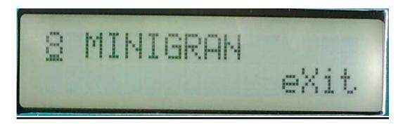
The minigran effect are a scaled down version of our deFormer's granulator effect. It cuts the input up in small fragments, and reorder these fragments to create a totally different sounding output. While the deFormers granulator works in sizes of 100 seconds, deMOON's minigran only works in sizes of milliseconds, so it is not very usable for rearranging beats. It's more like that it rearranges the waveform, and makes it sound glass/bell/voice-like or very strange.
