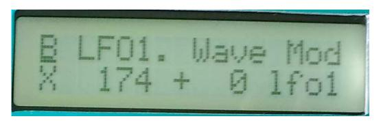
Edit 1: Oscillator LFO 1 waveshape. Value 0-255. 0: triangle, 64: saw, 128: square, 255: pulse.
