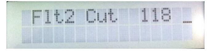
When a parameter MIDI controller are received, the parameter name and the received value shows in deMOON's display. To exit this, push the cursor(click)value.
