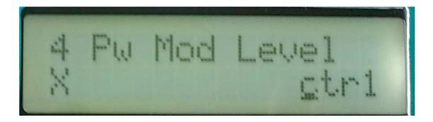
**Encoder – Pulse width modulation level source:** Selects a source, that modulates the level of the pulse width modulation. Choices are: manu(al) – nothing modulates the modulation level, lfo1, lfo2, env(elope), velo(city), osc(illator), ctr1, ctr2, ctr3.
