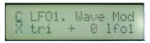
Edit 1: Filters LFO 1 waveshape. Value 0-255. 0: triangle, 64: saw, 128: square, 255: pulse.
