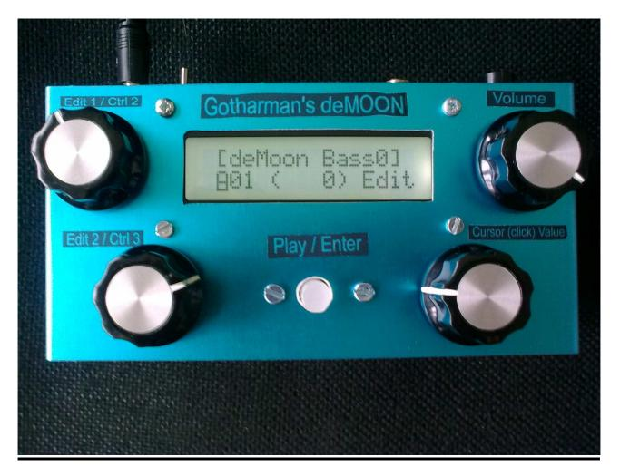
Edit1 / Ctrl 2: When on the pattern select screen (the screen showing on the picture) and on the edit page select screen, this knob transmits midi-controller 2 internally, and tweaks all parameters, which has midi-controller 2 selected as modulation source.
