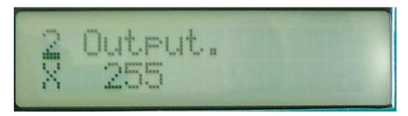
Edit 1 – Output level: Adjusts the final output level of the entire sound.
