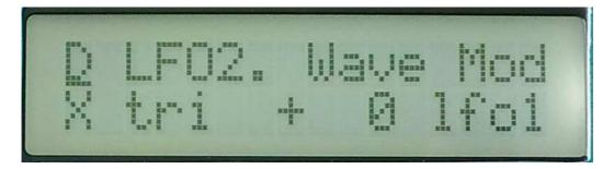
Edit 1: Oscillator LFO 2 waveshape. Value 0-255. 0: triangle, 64: saw, 128: square, 255: pulse.
