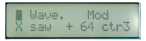
Edit 1 – Oscillator wave shape: Value 0 to 255, 0: triangle, 128: saw, 255: Square. If noise (on oscillator page 5) are any other value than off, 255 will be: noise instead of square.
