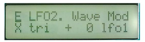
Edit 1: Filters LFO 2 waveshape. Value 0-255. 0: triangle, 64: saw, 128: square, 255: pulse.
