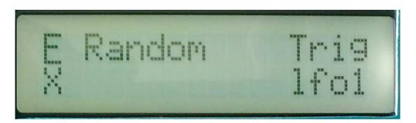
**Encoder:** Selects the filter random generator trigger source. Choices are: LFO1, LFO2, keyb (midi note-on's).
