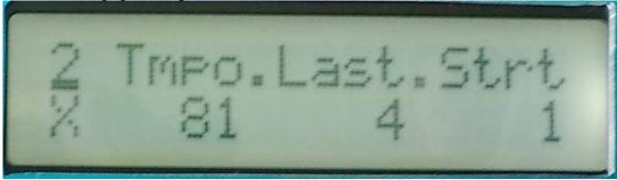
By placing the cursor under the number in the upper left corner of the display, and pushing the cursor(click)value encoder you can select among various edit pages in the selected edit group. By placing the cursor under the "X" and pushing the cursor(click)value encoder, you will exit to the edit page group select page.
