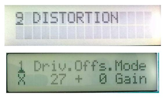
Edit 1 – Drive: Adjusts the gain of the distortion effect.
