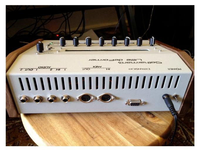
Connect the audio out 1 or 2 or both to a mixer or an amplifier, or anything else that ends out in a set of speakers, a single speaker, or even a pair of headphones, if you are in a neighbour friendly mood. Since it doesn't have build in speakers, it just needs to be connected to something, that can transfer its amazing sound to you.
