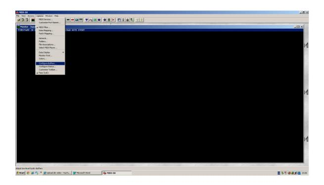
5. Enter the number "20000" in the "Bytes" box under "Low Level Output Buffers"
