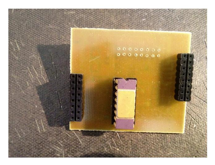
Mount the IG00156 chip in the socket. Take care that it is placed in the direction as pictured, and that the pins fits perfectly to the pins of the socket.
