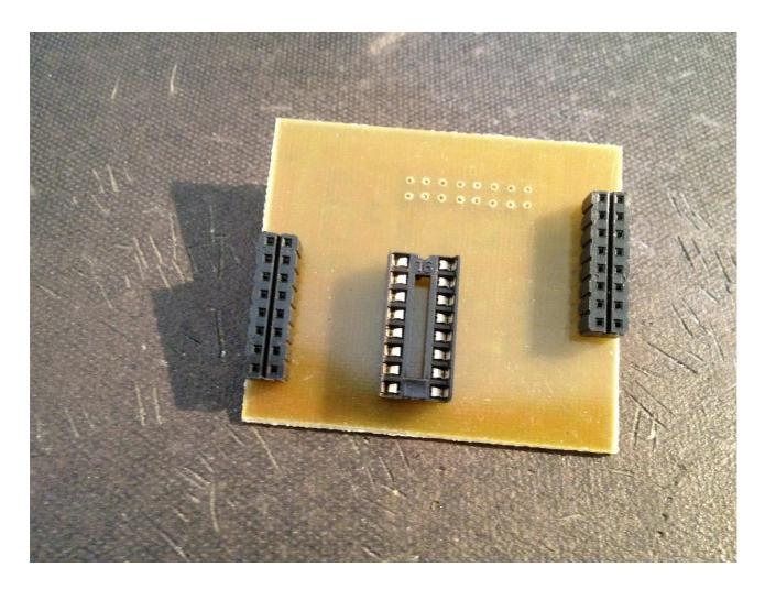
On the rear side of the small board, a socket is placed. This is for the IG00156 chip. Notice that in one end of the socket, there are a halfround hole. This has to match the same type of hole on the IG00156 chip.
