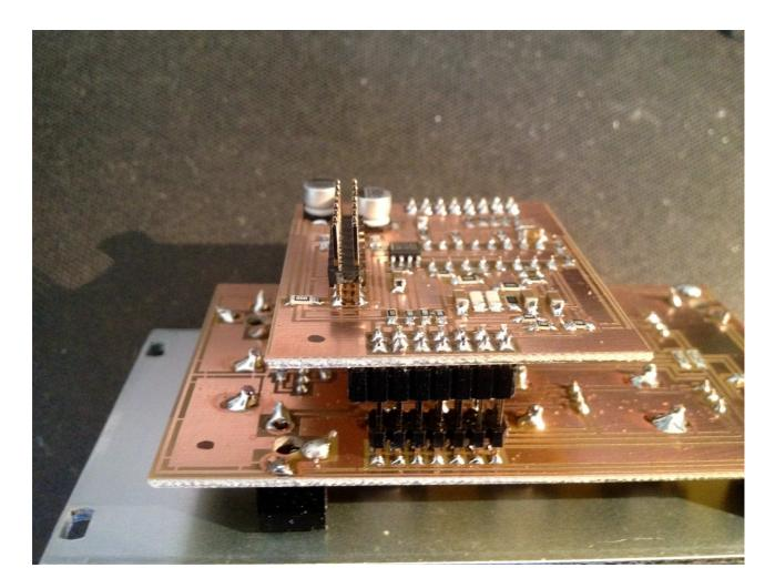
Mount the board again. Notice that in one side only 14 of the 16 connections of the header is used. It has to be placed like on the picture. On the other side all 16 connections are in use.
