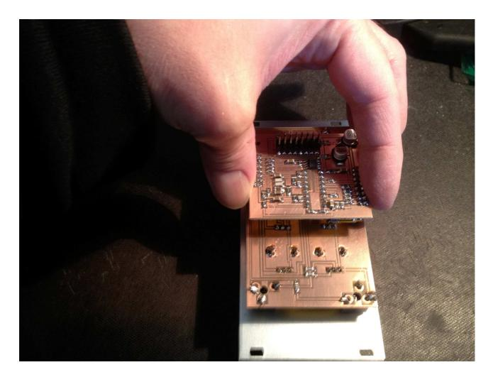
Remove the small board from the knob and jack board, using 2 hands.
