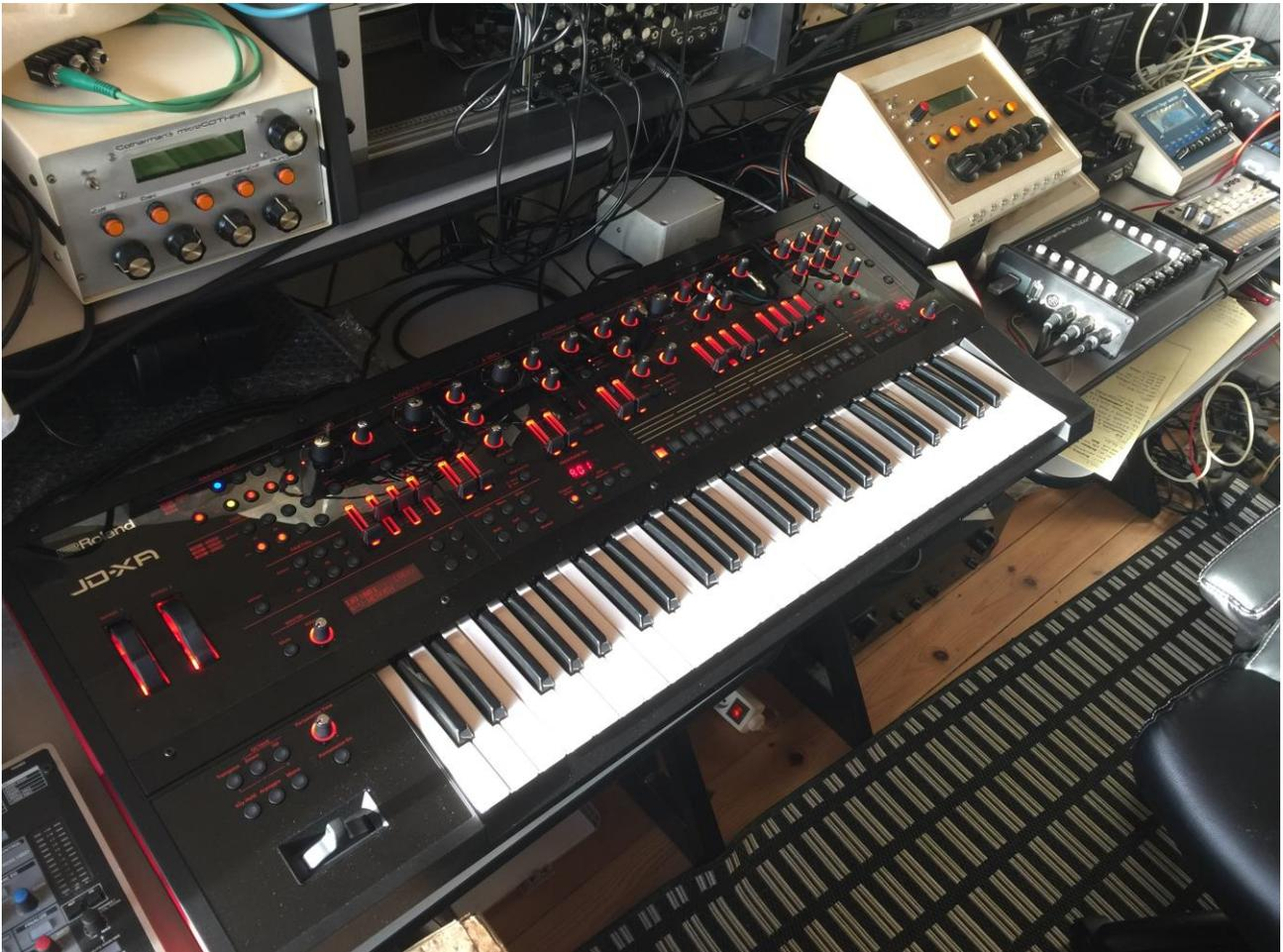
The Roland JD-XA transmits the same MIDI data on the channels of all its active parts, at the same time (i.e. note, bend and CC messages). This did not go very well together with Fuzion's channelizing system, so it now has an automatic MIDI filter system implemented, that will check for issues like this, and filter out any unnecessary MIDI messages.
