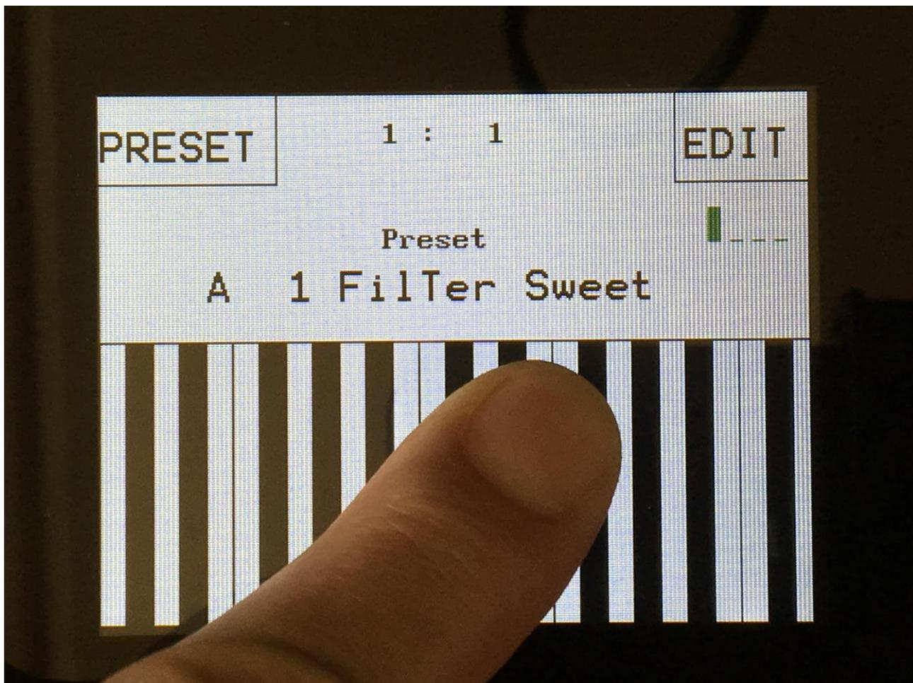
On the Preset and Song Select pages, it is, besides from playing notes on the touch keyboard, also possible to apply modulation to the sound, by placing your finger on different positions between the top and the bottom of the keyboard. This is referred to as Keyboard Y modulation. On any other pages, the keyboard only plays notes.
