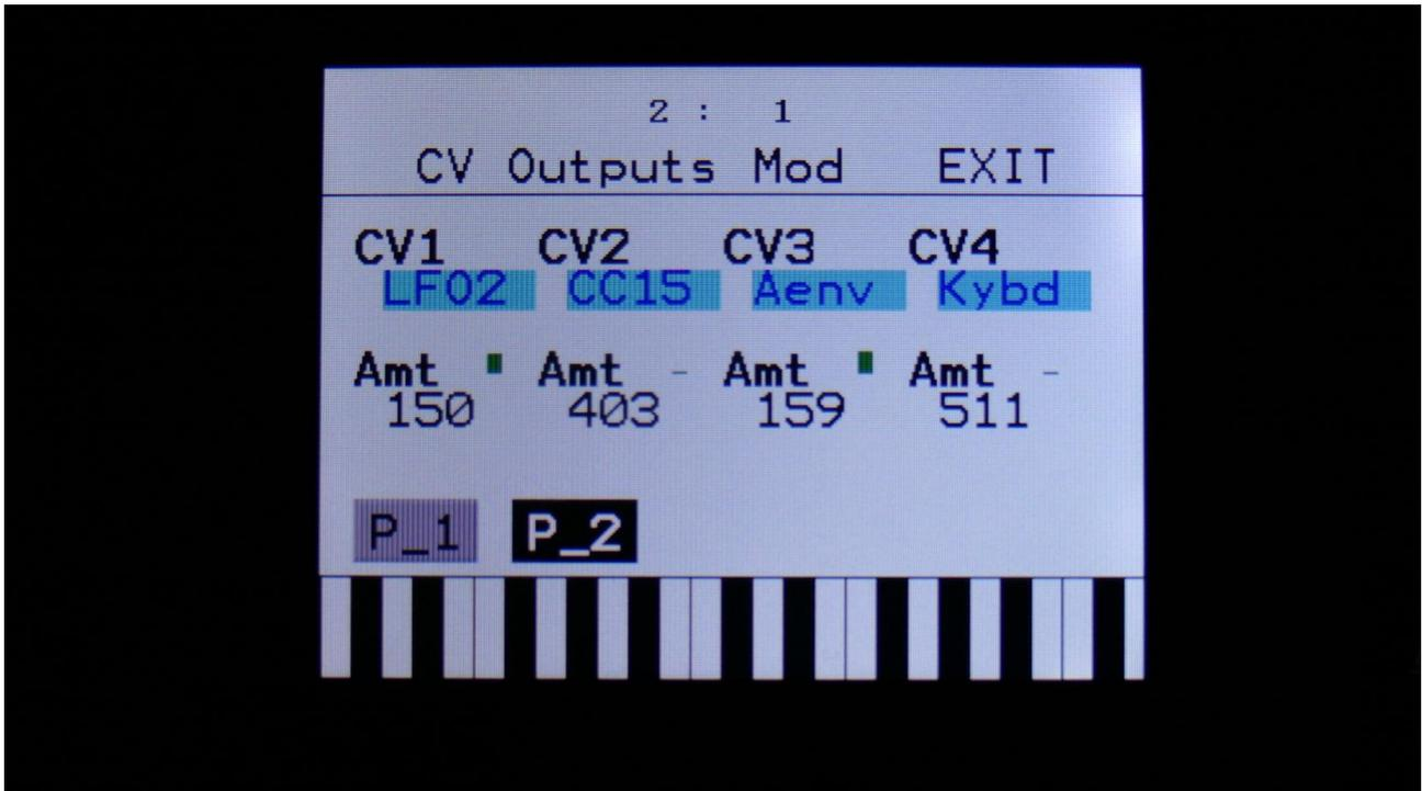
Here you can, with the upper row of parameters selected, by Edit Knob 1 to 4, select the modulation source for each CV output. For a complete list of modulation sources, see the list in the start of the synth section in this manual.
