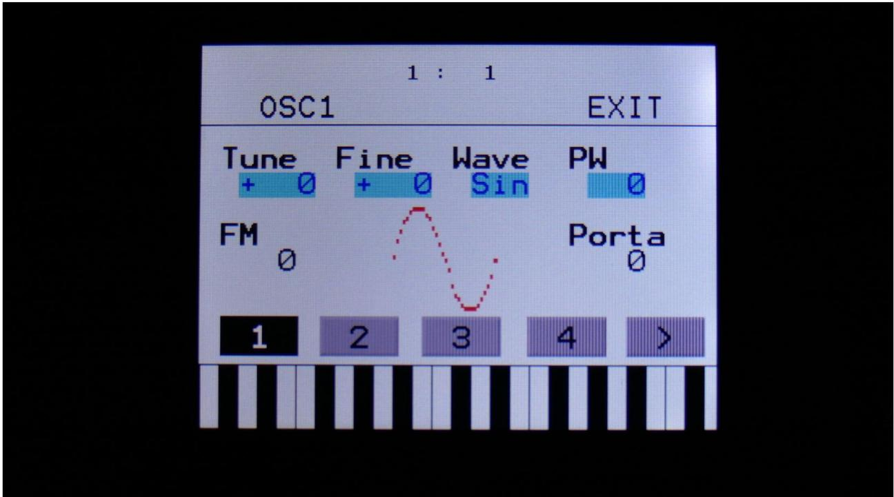
For Osc1 of each of the 4 Synth parts, it is possible to select if it should act as an oscillator or a sampler.
