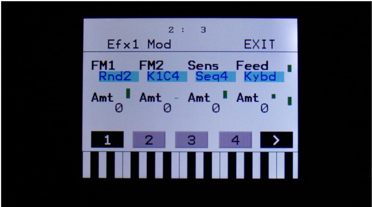
The 2 VU-meters at the right of the screen, shows the Effect input and output. The small VU-meters next to the parameters, shows the activity of the selected modulation sources.
