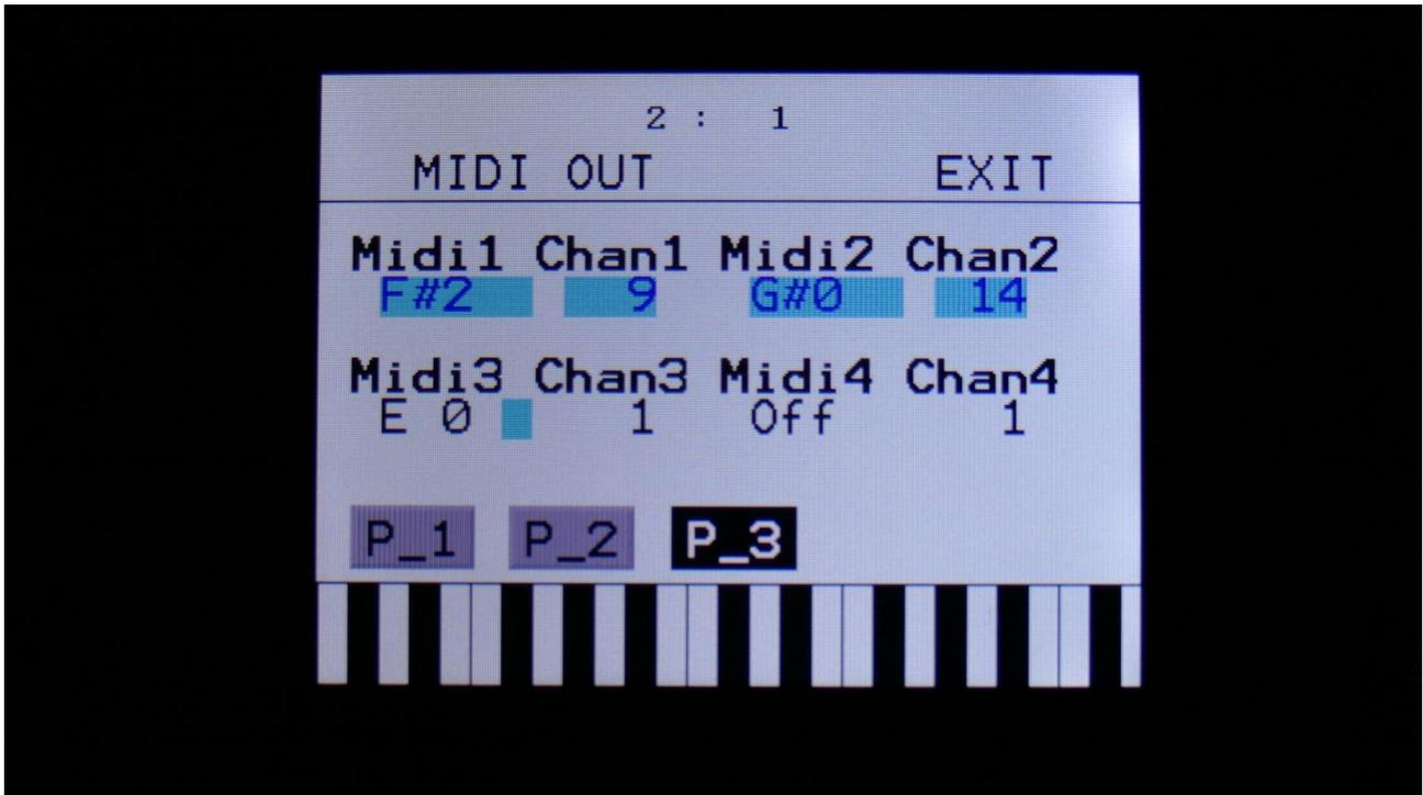
On this page it is possible to select a MIDI note number and a MIDI channel, that will be transmitted via MIDI out, when a trigger button is pushed. When a trigger button is set up to transmit a MIDI note, the sequencer track attached to that trigger, will also transmit MIDI notes on the same MIDI channel.
