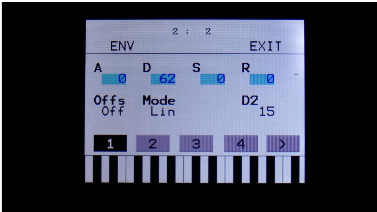
By touching the buttons numbered 1 to 4, the Envelopes's of part 1 to 4 is selected. In some play modes, it is not possible to edit all parts separately, and only the parts that can be selected, will be shown.
