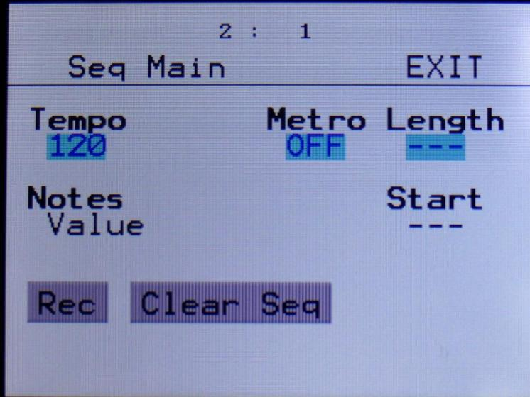
If the tracks lengths and start steps has been set up individually on each track, the global Length and Start steps will no longer be shown as a value, but just as 3 lines.
