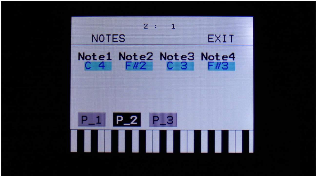
**Note1, Note2, Note3, Note4:** Sets the note number that each trigger button should send each of the 4 parts, when pushed. This setting only affects when the trigger buttons themselves are pushed, not when a trigger is controlled via MIDI, touch keyboard or sequencer.
