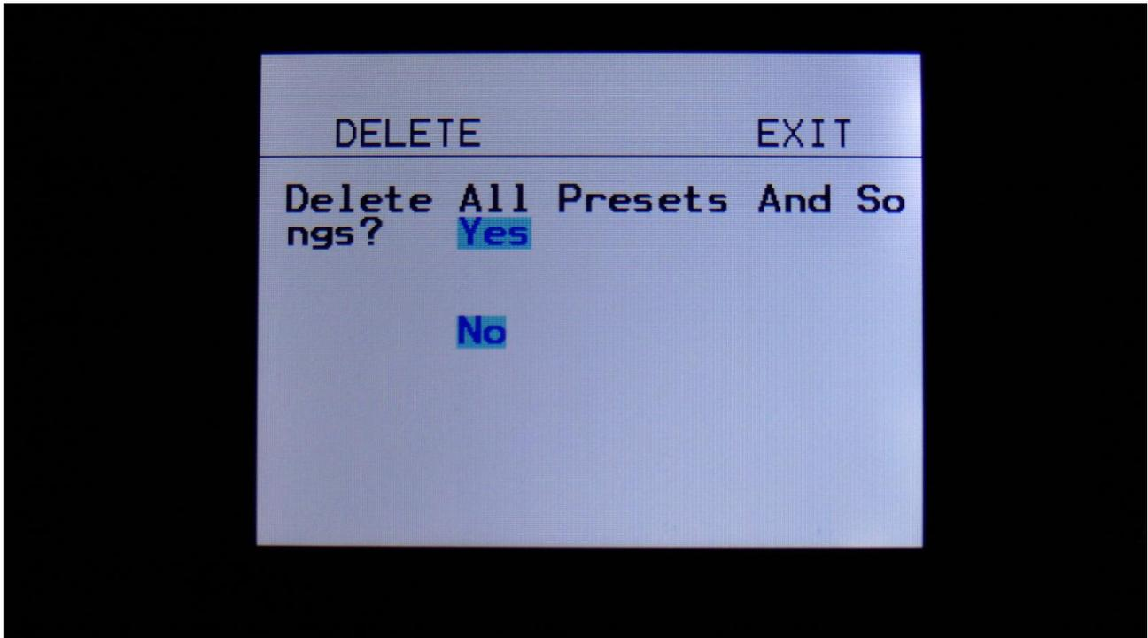
If you are really sure, that you absolutely have to do this, touch "Yes" to start the erase. All presets and songs will now be completely wiped out. While these are being erased, PolySpaze B's 5 button LED's will run a sequence. When the LED's shuts off, the erase has been done, and PolySpaze B will return to the More... screen.
