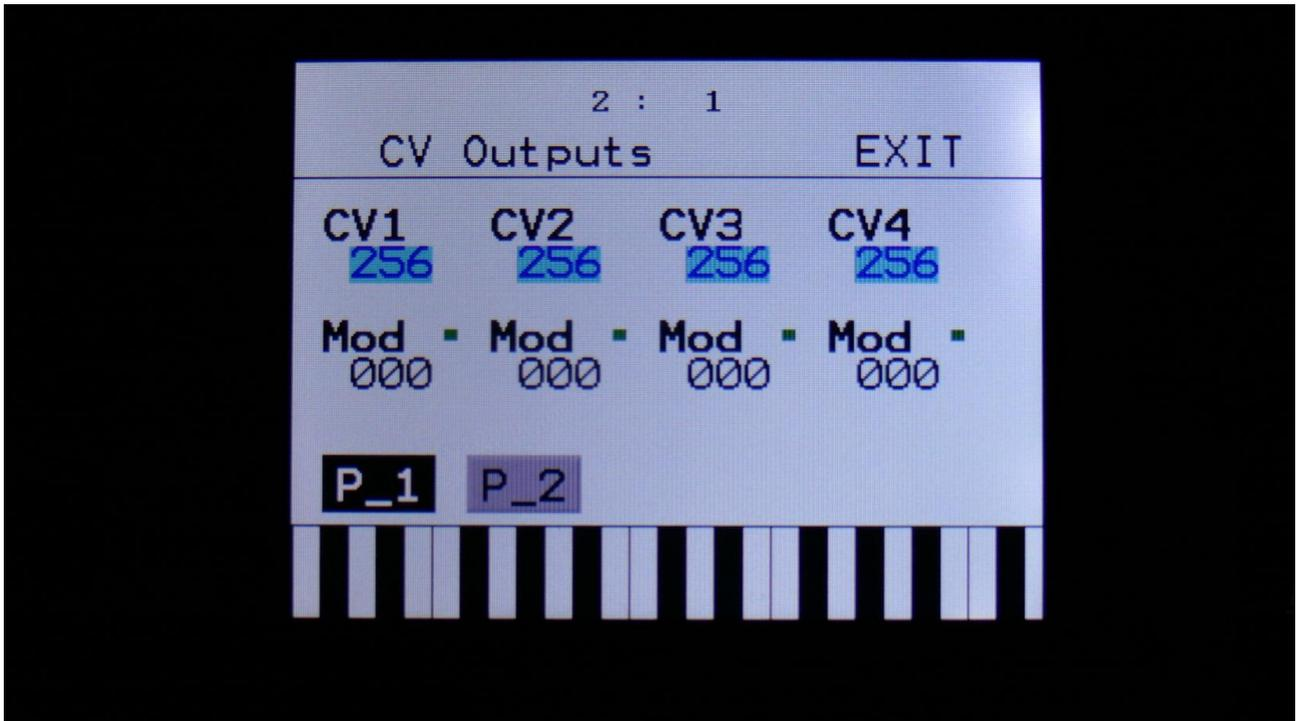
On this page, you can, with the upper row of parameters selected, by turning Edit Knob 1 to 4, set a static voltage to each CV output. This is useful, if you for instance, are controlling cutoff or resonance of an external filter, or tune of an external oscillator.
