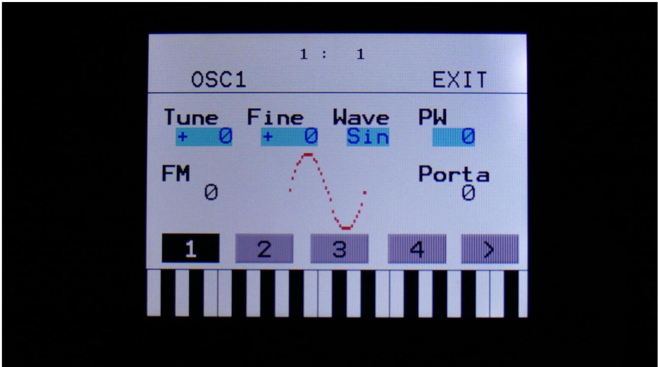
In the middle of the oscillator page, the current waveform is shown.
