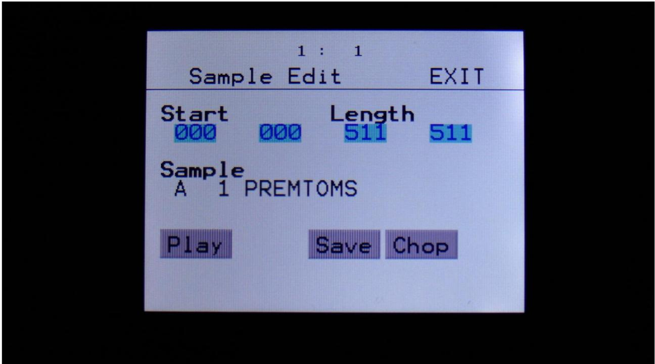
On this page you can audition samples from the FLASH memory, adjust the samples start and end points, and create sample chops.
