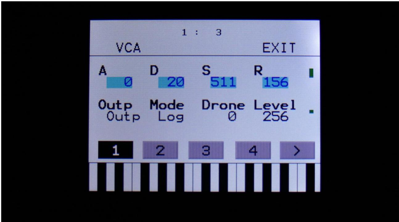
By touching the buttons numbered 1 to 4, the VCA's of part 1 to 4 is selected. In some play modes, it is not possible to edit all parts separately, and only the parts that can be selected, will be shown. Touch the arrow button, to enter other VCA pages, like Modulation.
