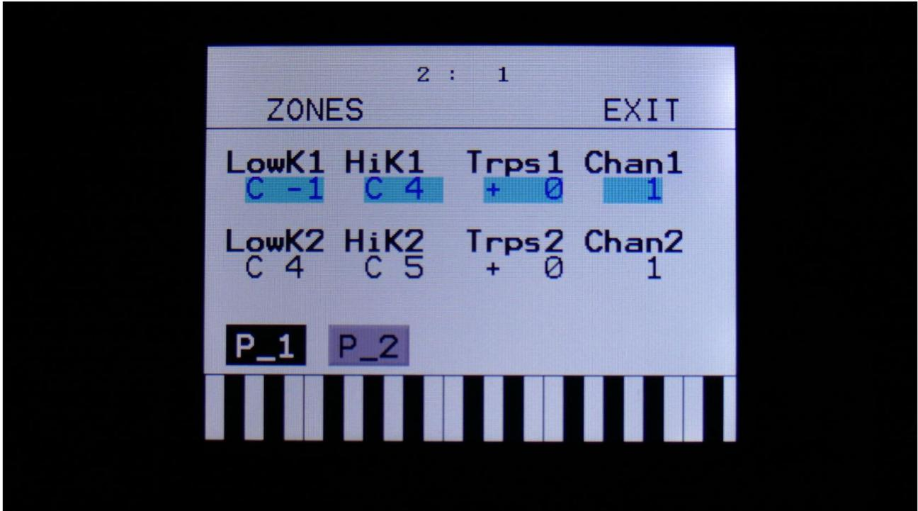
In this block you can set up the key zones and MIDI channels for each of the 4 Synth parts. These zones are effective only when PolySpaze B are in Multi-Timbral and MultiBank play modes, and are controlled from an external MIDI device or from the touch screen keyboard. It is also possible to transpose the incoming notes individually for each zone.
