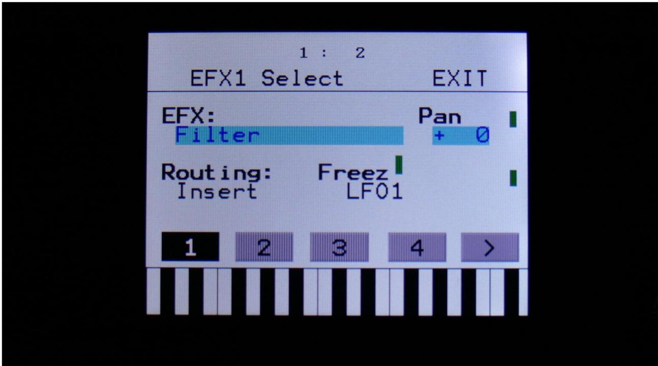
By touching the buttons numbered 1 to 4, the Effects's of part 1 to 4 is selected. In some play modes, it is not possible to edit all parts separately, and only the parts that can be selected, will be shown.
