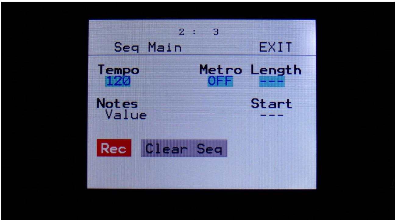
The Rec button turns red, when the Sequencer are in realtime record mode.
