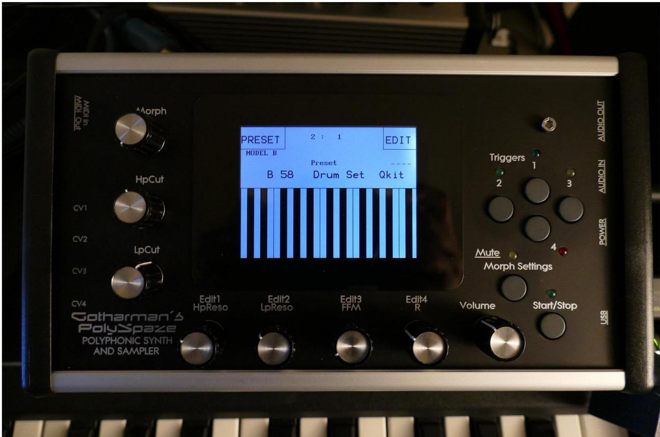
PolySpaze B has a highly sensitive capacitive touch display, 4 trigger buttons, a Morph Settings button and a Sequencer Start/Stop button. It has 4 Edit/Quick Edit Knobs for controlling and editing parameters and sending MIDI CC's, 2 additional Quick Edit Knobs, a Morph knob, and a volume knob.
