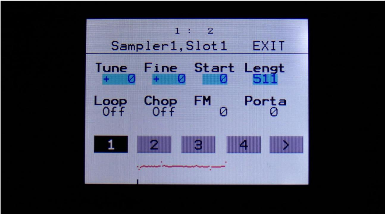
Each edit page has up to 8 parameters, that can be edited. The parameters are shown on the display as 8 parameter names, each with an alphanumeric value below them, that shows the current value of the parameter.
