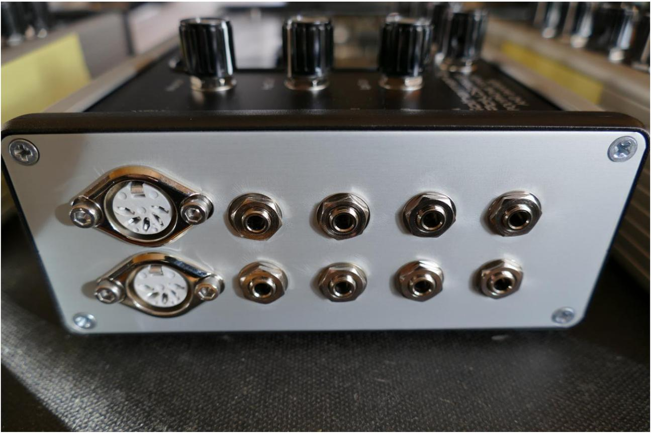
On the left end panel of your PolySpaze B, you will find the MIDI in and out connectors. The optional CV inputs and outputs are also found here, if installed. Please notice, that the upper row of CV connectors are the outputs, and the lower row are the inputs. The upper MIDI connector are the input, and the lower are the output.
