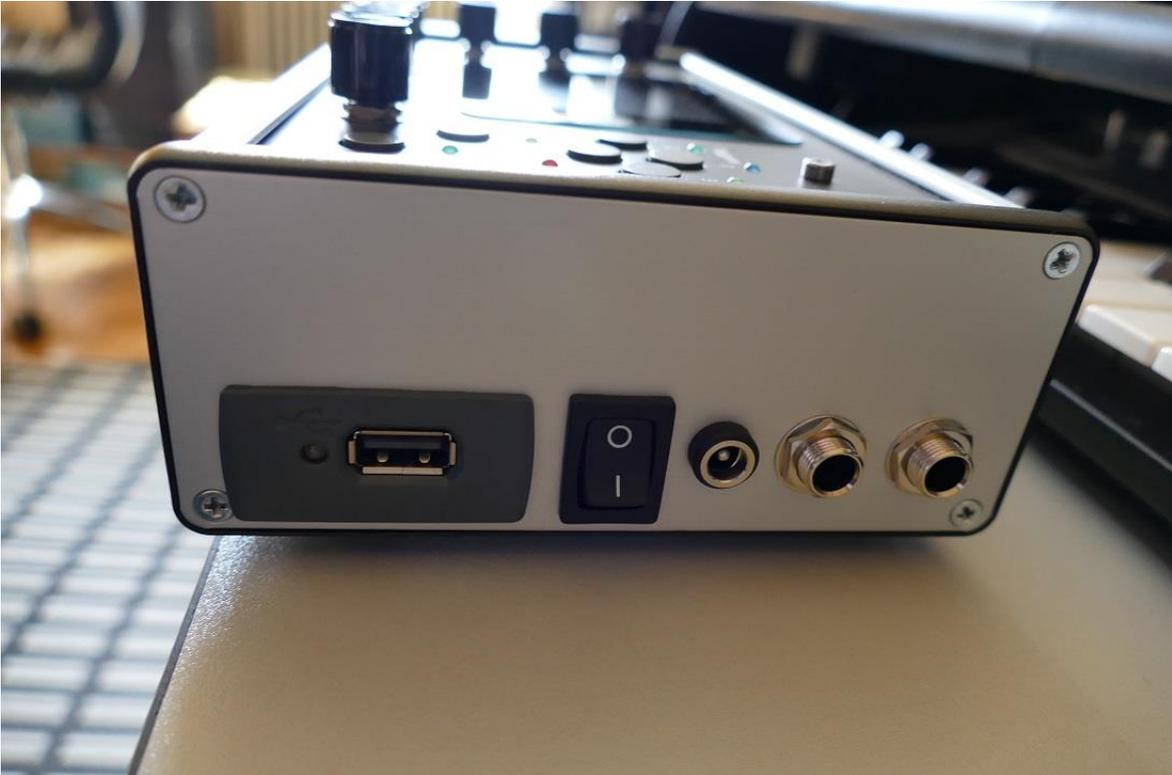
On the right end panel of your PolySpaze B, you will find the power switch, connection for power supply, stereo audio input and output, and USB. The audio inputs and outputs are stereo jacks.
