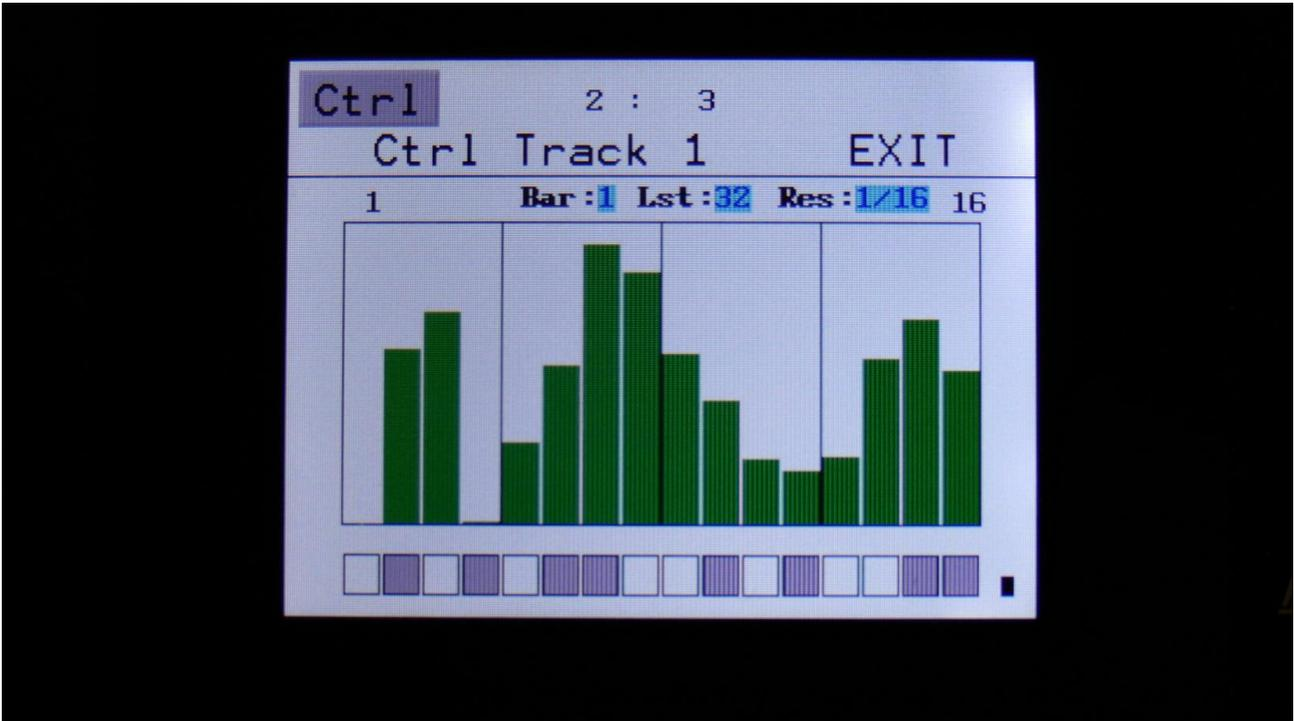
This will be the first page, you will enter, showing the controller value, that will be outputted for each sequencer step, when the sequencer is playing back. Here:
