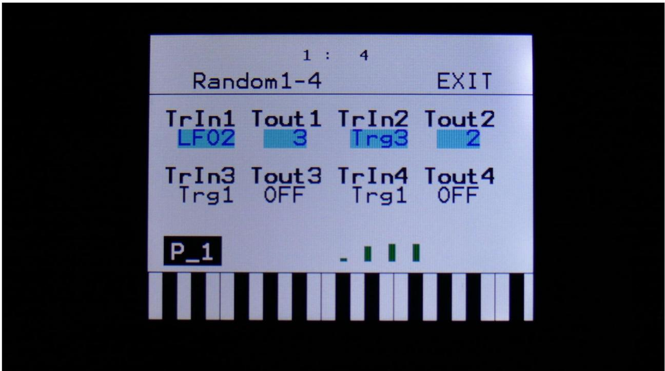
The 4 VU-meters at the bottom of the screen, shows the random generators outputs.
