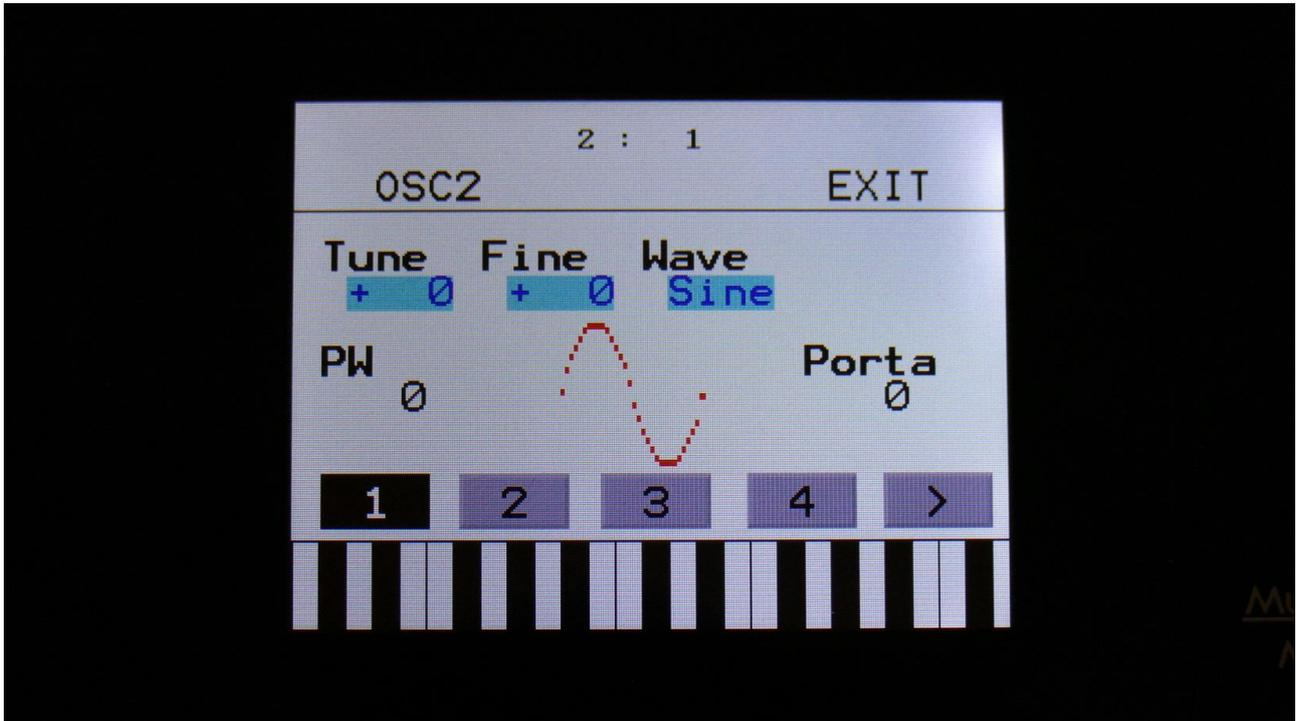
Oscillator 2 generates a waveform that is switchable between sine, triangle, saw, square and noise waveforms. It is also possible to select any of the 2 audio inputs as the audio source, instead of Osc2, if you wish to route the audio inputs through PolySpaze B's filters and effects. Pulse width are adjustable for sine, triangle, saw and square. Pitch and PW can be modulated. The pitch range of the oscillators are chromatically over the entire 10 octave MIDI keyboard range.
