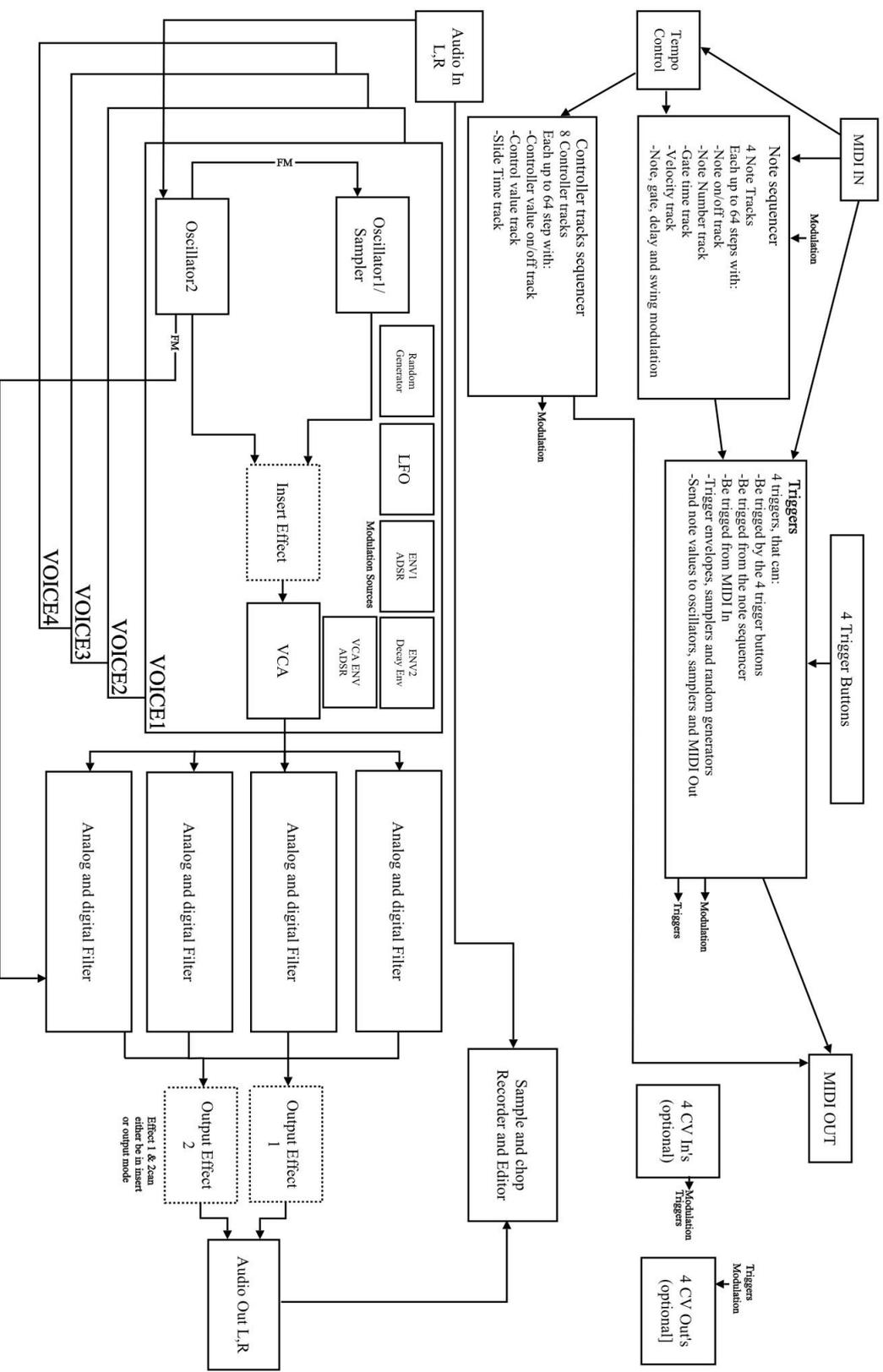
Gotharman's PolySpace B Structure in PolyBank Mode and Multi-Bank Mode
