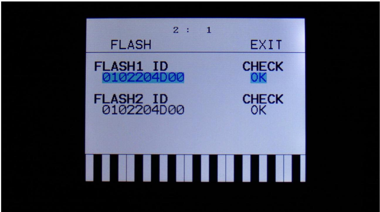
This page should look exactly like on the picture (except for the touch screen keyboard). If it doesn't, the FLASH memory on your PolySpaze B might be defective, and should be replaced. Please get in touch with Gotharman's regarding this.
