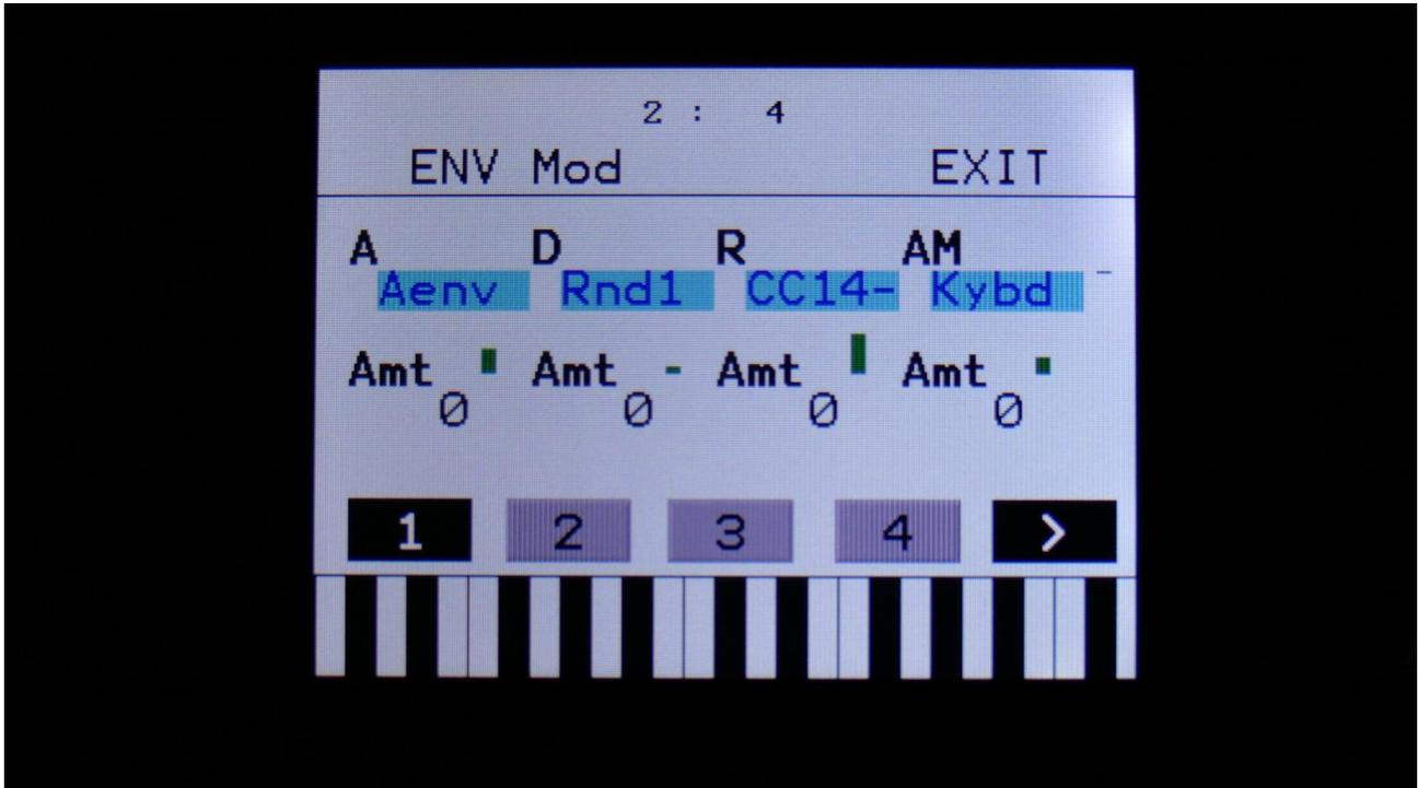
The VU-meter at the right of the screen, shows the Envelope output. The small VU-meters next to the parameters, shows the activity of the selected modulation sources.
