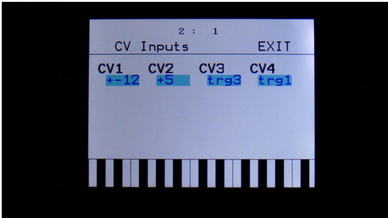
Here you can, by turning Edit Knob 1 to 4, set up each CV input. The possibilities for each input are:
