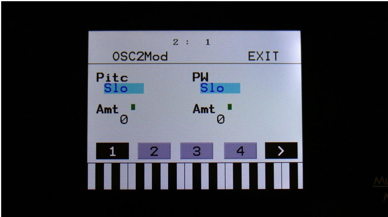
The small VU-meters next to the parameters, shows the activity of the selected modulation sources.
