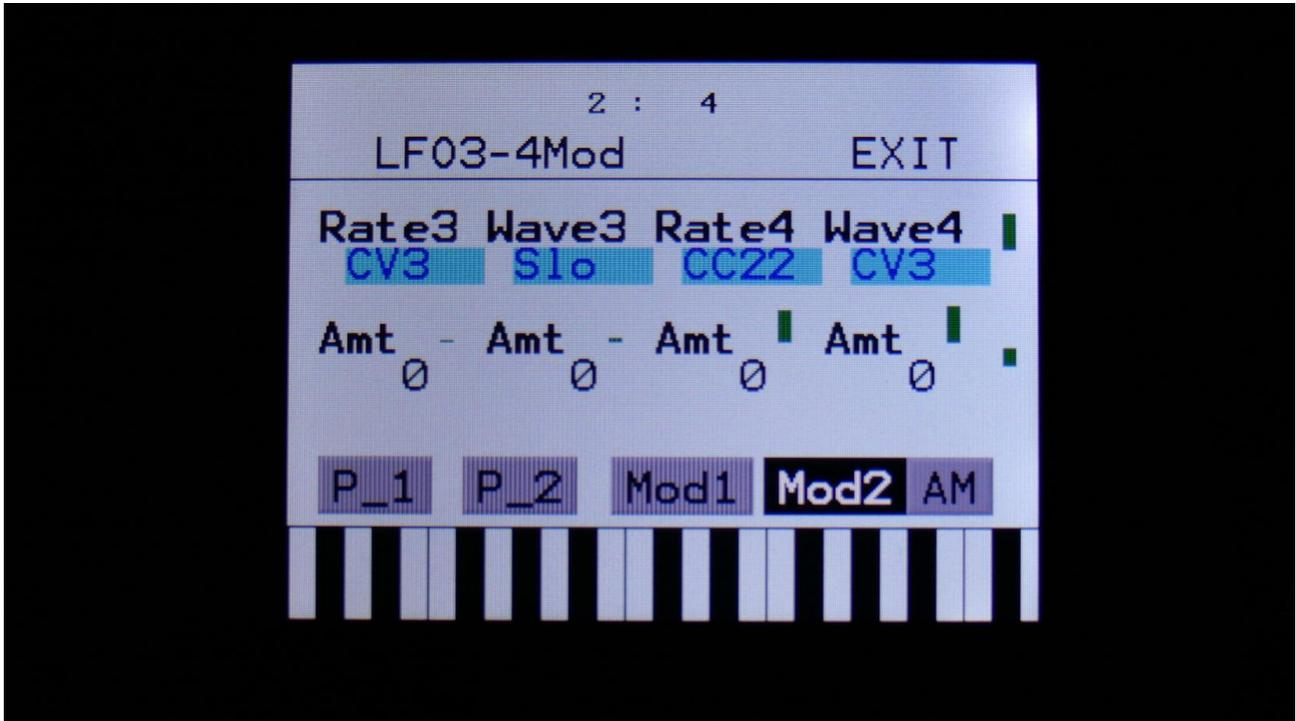
The 2 VU-meter at the right of the screen, shows the LFO outputs. The small VU-meters next to the parameters, shows the activity of the selected modulation sources.
