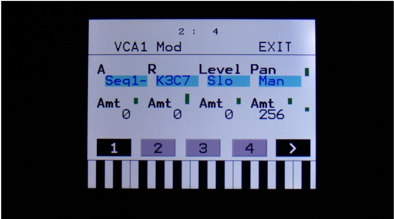
The 2 VU-meters at the right of the screen, shows the VCA input and output. The small VU-meters next to the parameters, shows the activity of the selected modulation sources.
