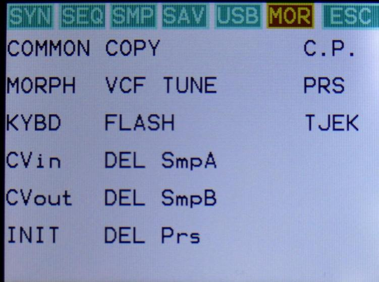
This will get you to the More... page. Here you can set up all the basic PolySpaze B things, like MIDI channel, morphing, touch keyboard and CV in's/out's, make the analog filter tune, check and erase the PolySpaze B memory, initialize the preset and change to song mode.
