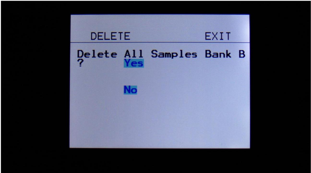
If you are really sure, that you absolutely have to do this, touch "Yes" to start the erase. The sample bank will now be completely wiped out. While it is being erased, PolySpaze B's 5 button LED's will run a sequence. When the LED's shuts off, the erase has been done, and PolySpaze B will return to the More... screen.
