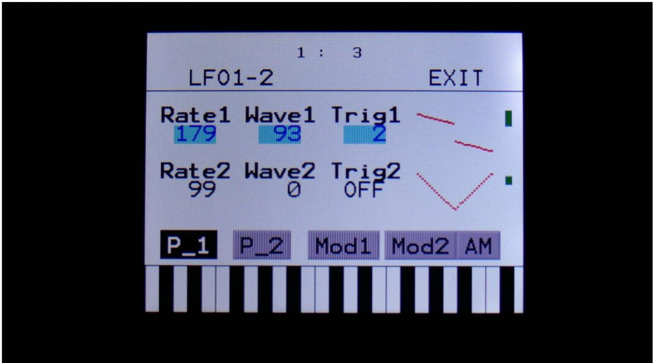
To the right on the LFO page, the current waveforms are shown. The VU-meters at the right of the screen, shows the LFO outputs.
