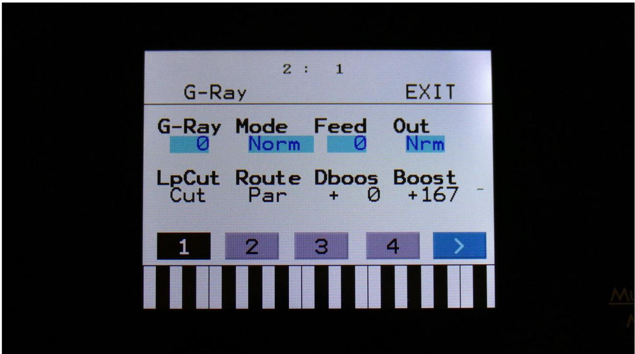
**G-Ray:** Adjusts the amount of g-RAY intermodulation. 0: no g-RAY, 3: max g-RAY. Range: 0 to 3.
