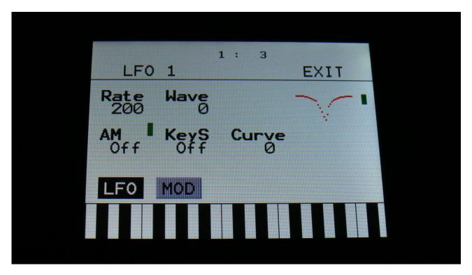
When the Curve parameter is set to 256, the LFO will output a linearly shaped triangle wave, just like it did before the Curve parameter was added:
