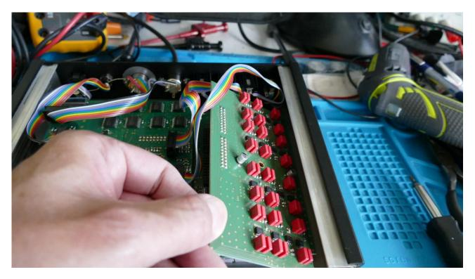
Lift the side of the filter board, which is pointing towards the middle of the casing, up a bit, and take the board out.
