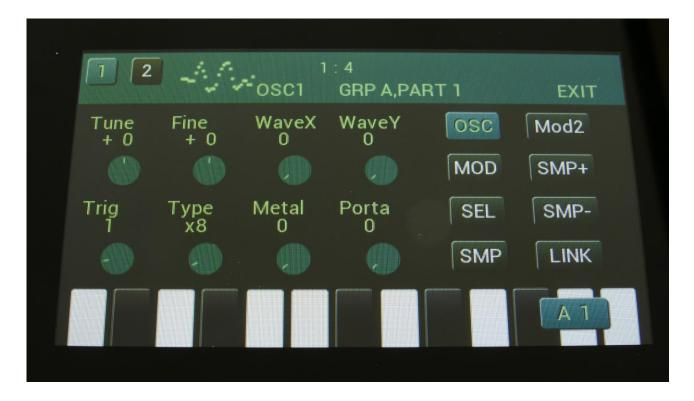
Each group has 2 of these oscillators (8 in total), which can run in several different modes, for maximum flexibility. The outputs of the oscillators can be connected to any audio and modulation inputs. To select a specific oscillator, first select the group/part, and then touch the numbers in the upper right corner.
