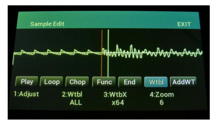
On the graphical sample edit page, with the sample, which you would like to build a wavetable from, selected, touch the Wtbl button, so that this turns blue. Zaturn will now create one wave for a table, consisting of 512 sample points, equally spaced between the selected start and end points. As soon as Wtbl mode is switched on, the currently generated wave will be audible.
