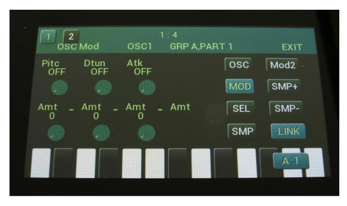
The MOD page, when Perc, Prc2 or Prc3 is selected as Type
