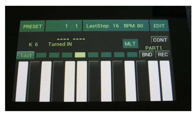
On the Preset and Song Select pages, it is, besides from playing notes on the touch keyboard, also possible to apply modulation to the sound, by placing your finger on different positions between the top and the bottom of the keyboard. This is referred to as Y modulation. On any other pages, the keyboard only plays notes.
