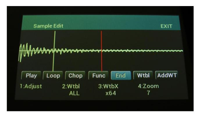
By touching the End touch button, so that it turns blue, the screen will now be focused on the end point, which is indicated as a vertical red line. When you touch the screen now, the red line will move, indicating that the end point is selected. It is also possible to change the end point, by rotating Edit Knob 1.
