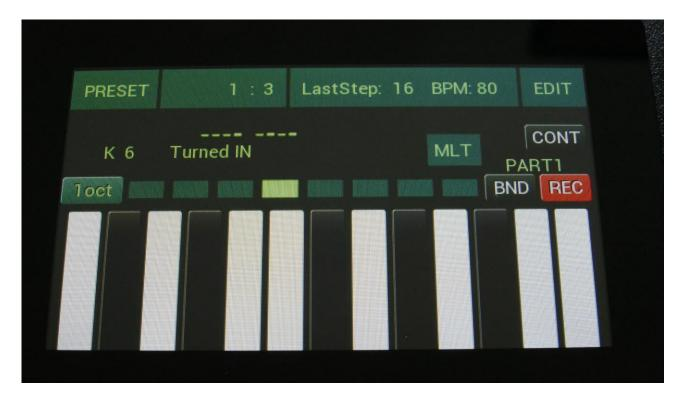
Zaturn will now show the Preset select page. The REC indicator on the preset select page, has now turned red, indicating that Zaturn is in recording mode. Song realtime recording can also be switched on or off, by touching the REC indicator.
