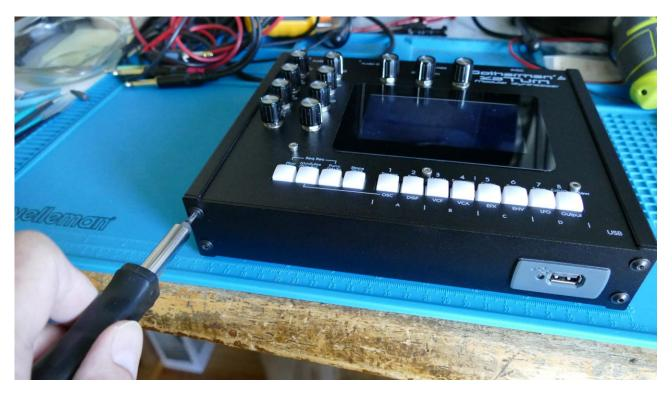
Remove the 4 hex screws, located on the front facing panel, using a T10 Torx. Place the screws in a safe place.
