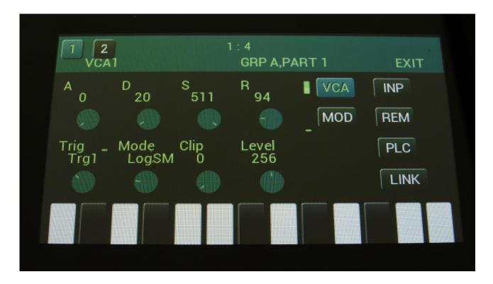
Each group of Zaturn has 2 VCA's (8 in total) with built-in ADSR Envelopes and an envelope Clip parameter, that adds more punch to the VCA. The VCA's has 16 different linear and logarithmic modes (characteristics), and the envelope time can be timed by 4, for long envelope times. The VCA envelopes can be trigged by any sources. The A, D, R and output level parameters can be modulated.
