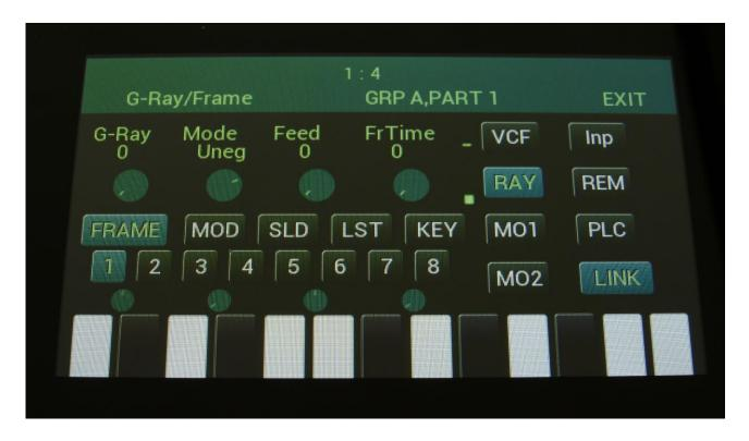
With frame one still selected, you might now want to adjust the frame 1 time, using the **FrTime** parameter, and to touch the **SLD** (Slide) button, to make the frame sequencer slide smoothly from frame 1 to frame 2.
