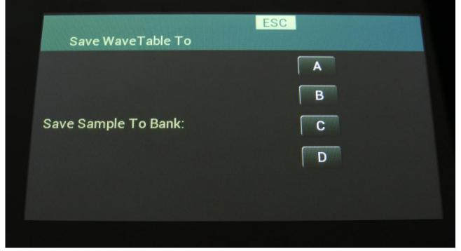
Select the sample bank, on which you would like to save the wavetable to, by touching the A, B, C or D field. 18 min. and 43 min. Zaturn's only has Bank A.
