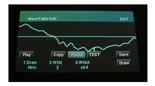
At any time under this process, it is also possible to test the wavetable. Touch the TEST button, so that this turns blue.
