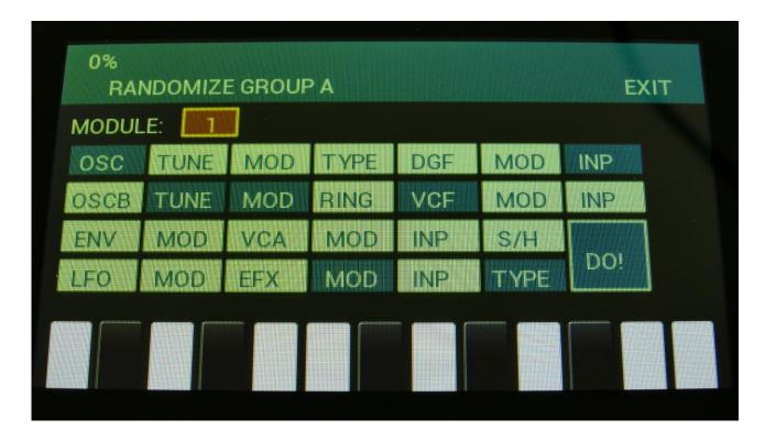
First, make sure that you have selected the right group, in which you want to randomize the parameter values. You can do that, by pushing and holding the Steps/Part button, while pressing one of the 8 step buttons. The selected group is shown at the top of this page.
