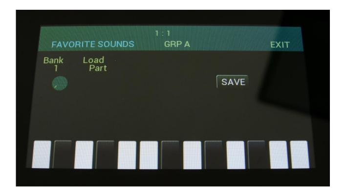
When on the favorite sounds page, pushing a step button will load a sound to the currently selected Group, while playing the sound back for auditioning, and showing the preset and group location on the display. Step buttons that has a favorite sound stored, will light up.
