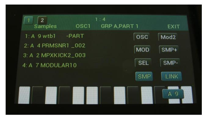
Here you can select 4 samplings for the part. The number of these samplings, that are used, is set by the #Smp parameter on the SEL page. The 4 samples can be selected to play back, setting the Chop parameter, and by chop select modulation. To select a sampling for any of the 4 slots, simply touch the sample name. Now this page will pop up:
