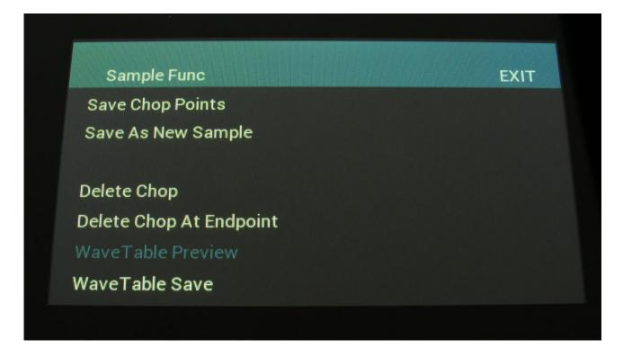
Touch **WaveTable Preview**, so that this turns blue. Now you will hear your wavetable playing back. Adjust **Edit Knobs 1 and 2**, to scan through the waves (**Edit Knob 2** is only active at 64 waves). When you are satisfied with the result, touch WaveTable Save, to save your new wavetable. Now this page will appear:
