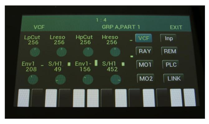
Adjusting the Cut and Reso parameters on the VCF page, when the filter is in Frame Sequencer mode, will set an offset for these parameters, affecting all filter frames at the same time.
