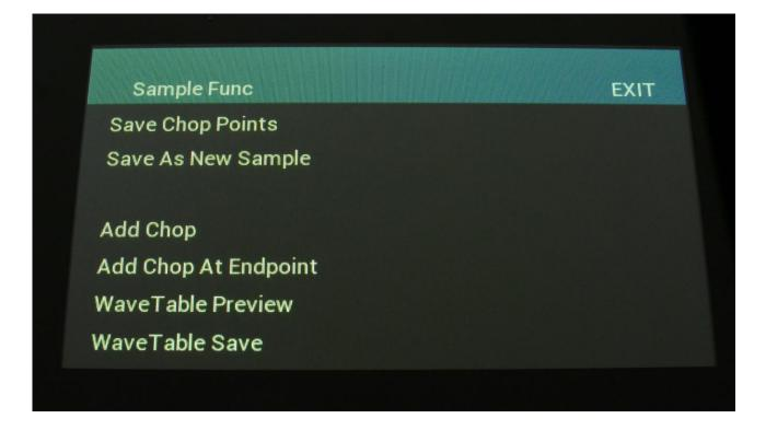
Touch "Save As New Sample". A new page will now open. Select the sample bank, that you would like to copy the sampling/portion of the sampling to, by touching the A, B, C or D touch button.
