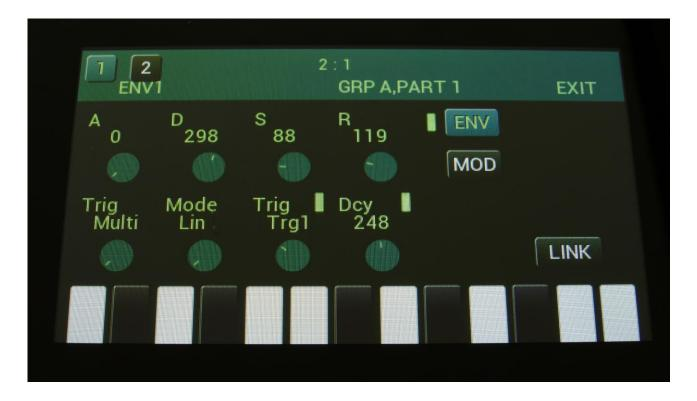
Each group has 2 envelope modules (8 in total), each with an ADSR envelope and a Decay envelope. The ADSR envelope can run in various linear and logarithmic modes, the envelope time can be timed by 4, for long envelope times, and the ADS segment can be looped. The envelopes can be trigged by any sources. The A, D, R and output amount parameters can be modulated. The extra decay envelope, is always linear. When the ADSR Envelope is looped, the Decay envelope is looped in sync with this.
