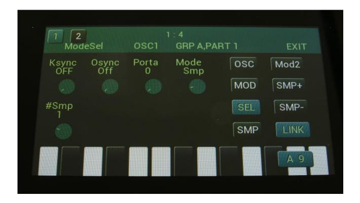
Set the Oscsillator in sampler mode, and touch the SMP touch button to select the sampling, that you just wave chopped (or any other sampling that you have wave chopped).
