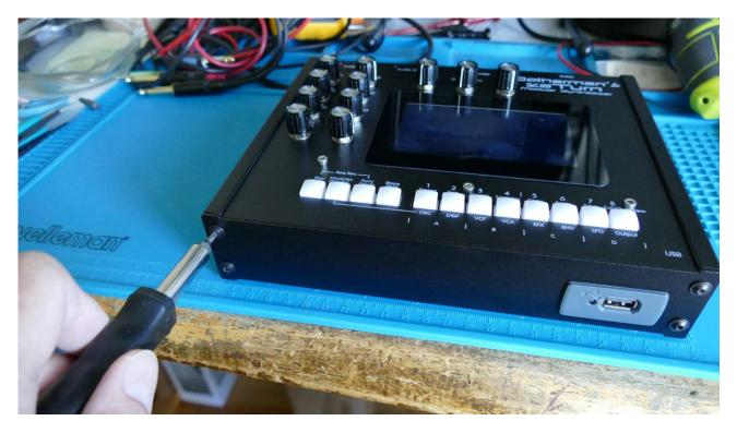
Turn zaTurn over and mount the hex screws. You will need to hold the end panel in place, when you are mounting these screws.
