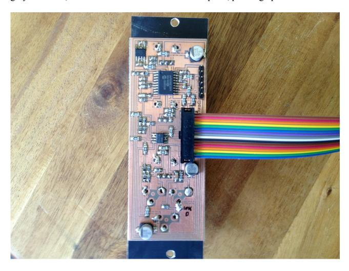
Mount the other end of the power cable to the powerboard of your Eurorack case. Make sure, that pin 1, the brown core, is connected to −12 volt. Mount Windy in your Eurorack case, using screws.
