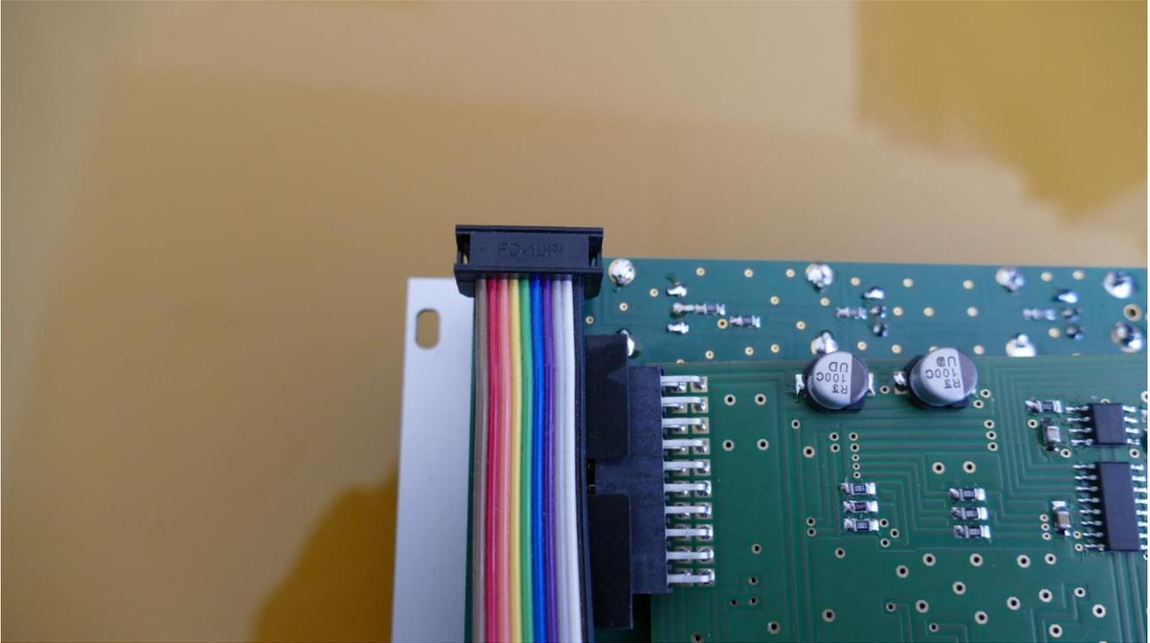
Connect the power cable with the brown cable (-12V) facing upwards, if it is a multi-colored cable, or the red line facing upwards, if it is a grey cable.
