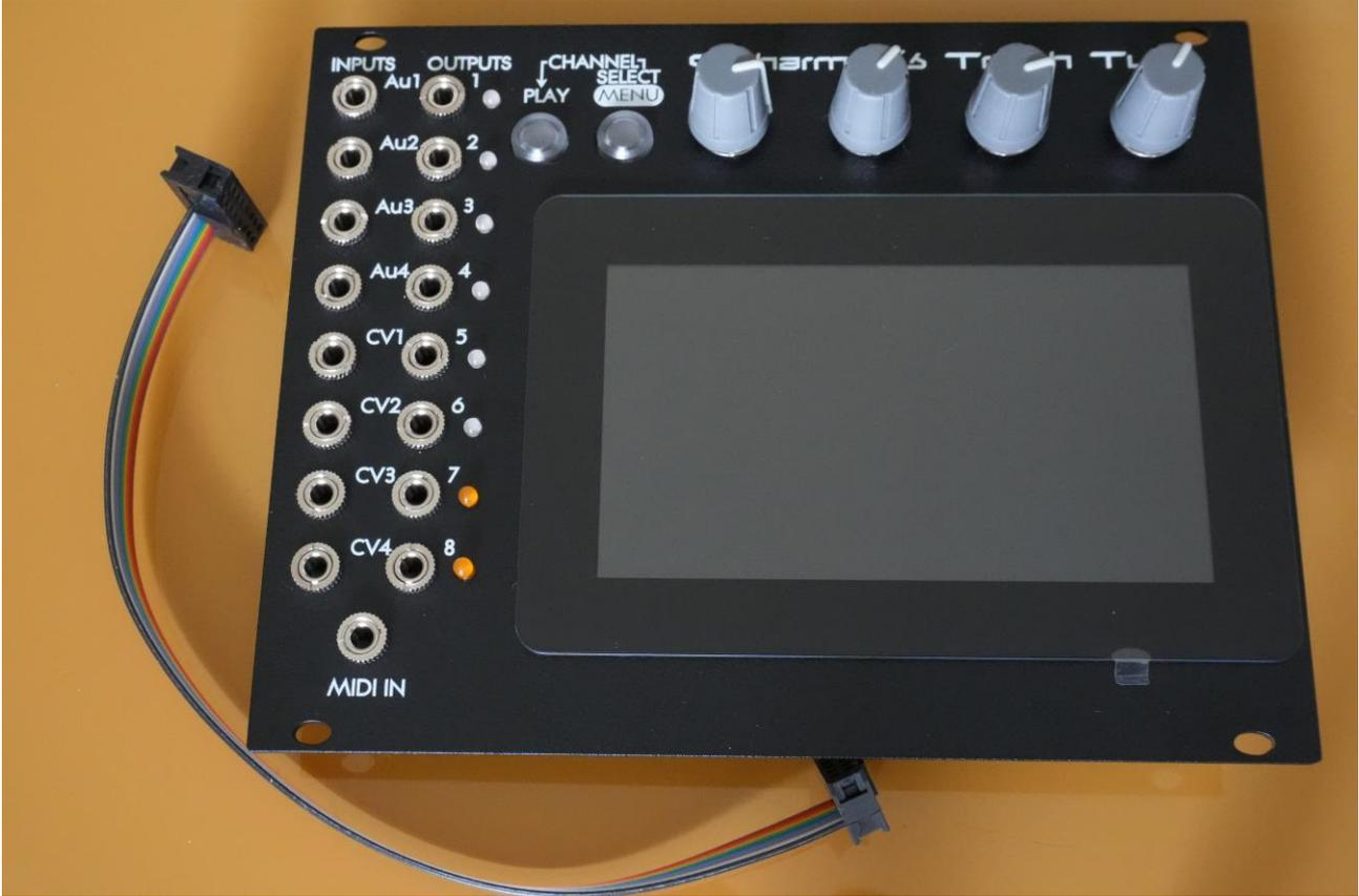
The power cable is usually attached to Touch TuuL, but if it should become detached, it should be placed with the brown line pointing towards the “-12V” print.
