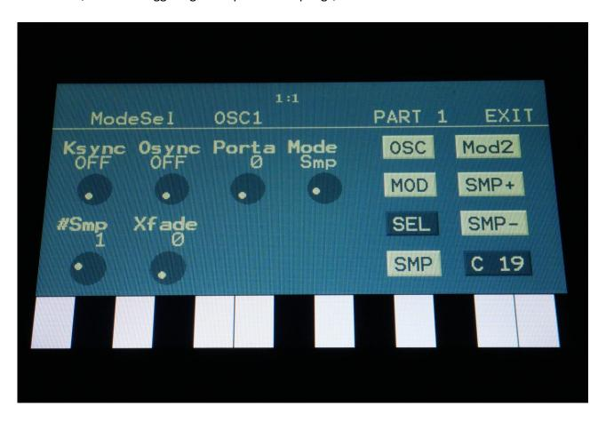
These clicks can now be dampened or even be removed, by turning up the new Xfade parameter, found on the OSC SEL page.
